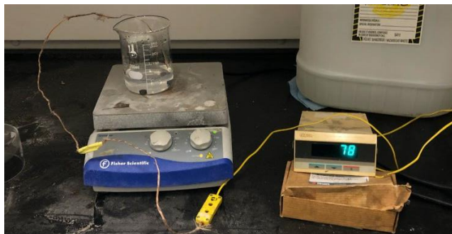
Figure 4.1: Initial experiment with beaker, hot plate, and thermocouple.
