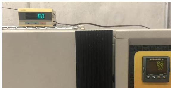
Figure 3.4: Oven maintained at 80°C when set to 88°C.
