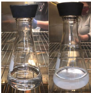
Figure 5.12: P-5 at beginning and end of 72-hour oven experiment showing successful H_2O_2 retention.
