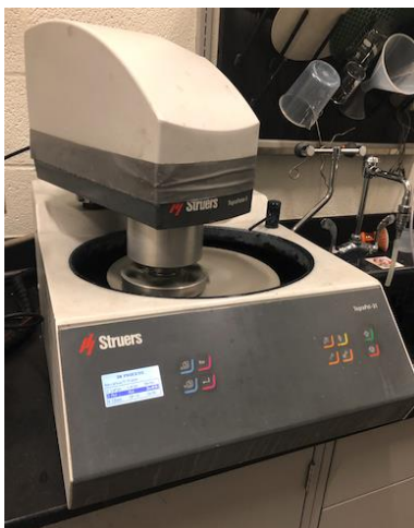
Figure 3.1: Struers TegraForce-5 used for ground and mirror polish finish on plates.
