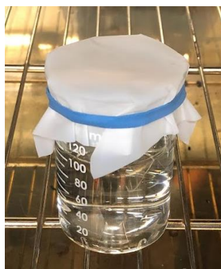
Figure 5.28: Batch P-14 in oven prior to 12 hours with PTFE cover.
