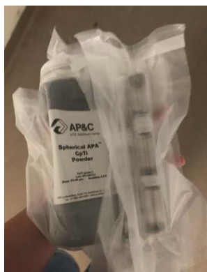
Figure 5.3: CP-Ti powder separated and resealed.
