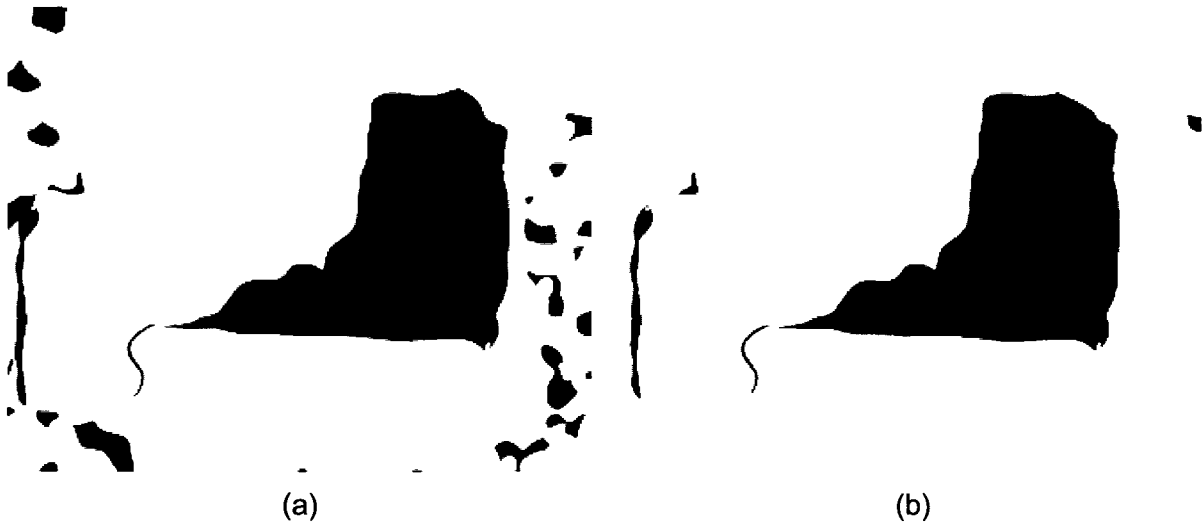
Figure 4.20. Partition masks computed (a) without and (b) with minimum threshold, where black represents the region of interest.
