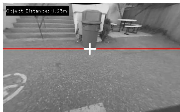
Figure 7.2: The true object distance is established by manually indicating its base. Using the knowledge of the camera's orientation, height and intrinsics, the indicated pixel (white crosshair) is projected to the world ground plane.
