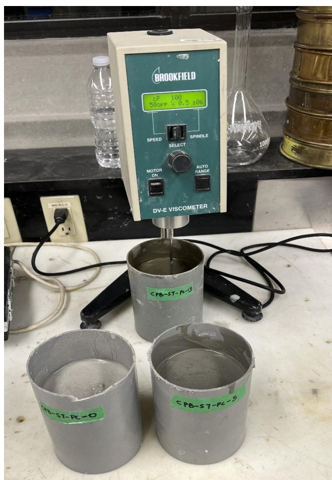
Figure A-3: Testing Apparatus-Brookfield digital viscometer (DV-E model)
