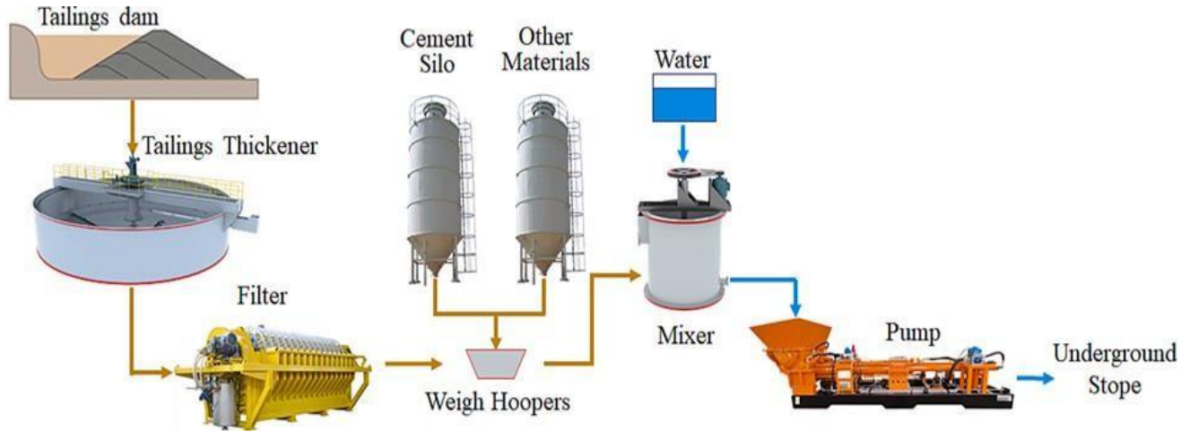
Figure 5: Typical layout of CPB plant (Fang et al., 2023).
