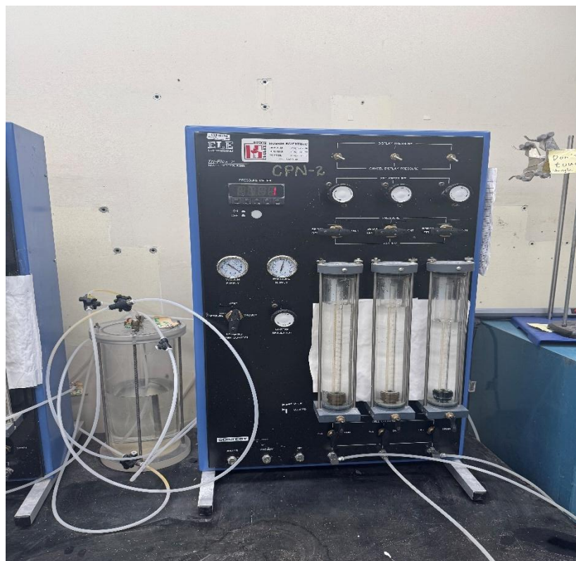
Figure A-5: Testing Apparatus- Tri-Flex 2 flexible wall permeameter
