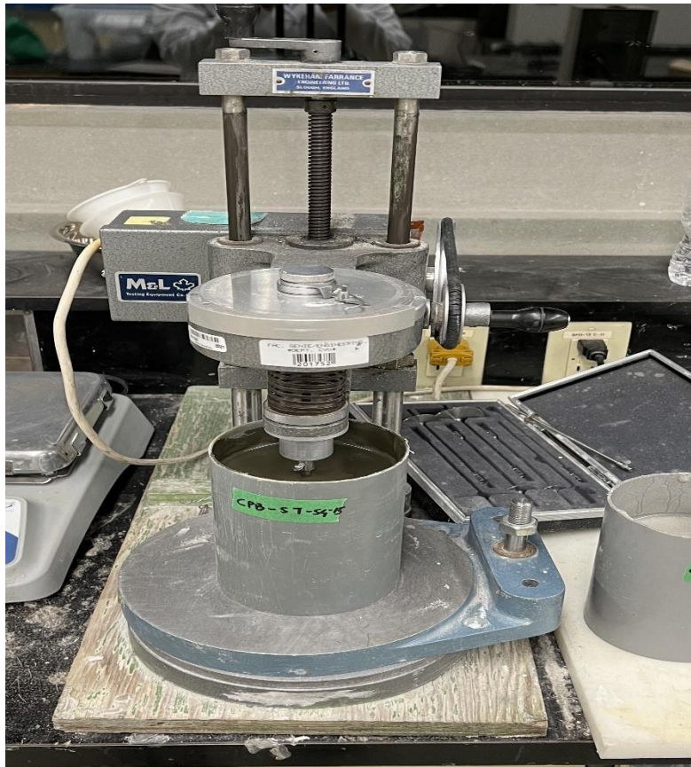
Figure A-4: Testing Apparatus-Wykeham-Farrance laboratory vane shear device
