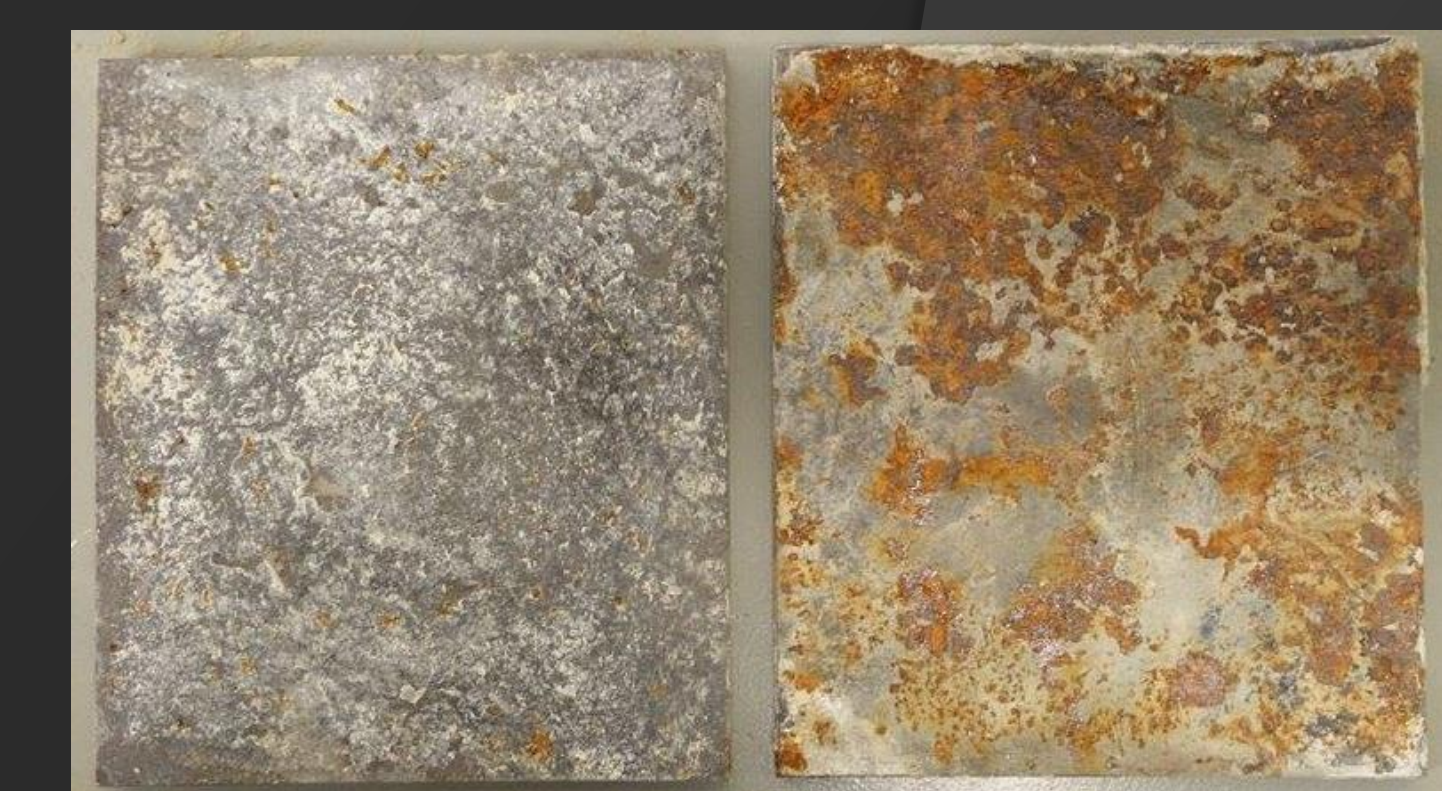
Fig. 10: Steel plate for non-corroded and corroded samples
