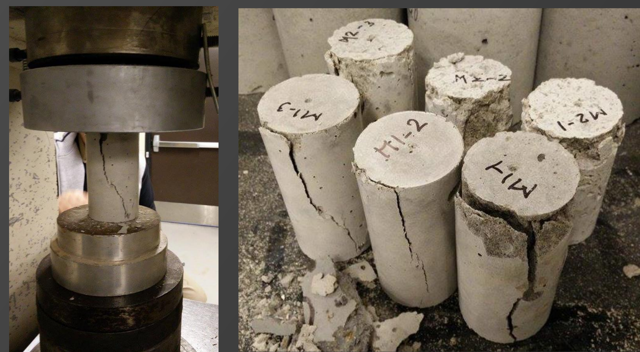
Fig. 4: Cylinder samples during and after test
