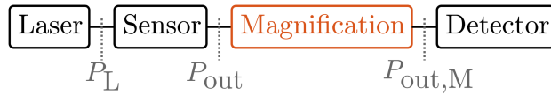
Figure 3.13: Conceptual setup for all-optical signal magnification. P_L is the laser power, P_{\text{out}} is the power at the output of the sensor, and P_{\text{out},M} is the magnified sensors' output power.
