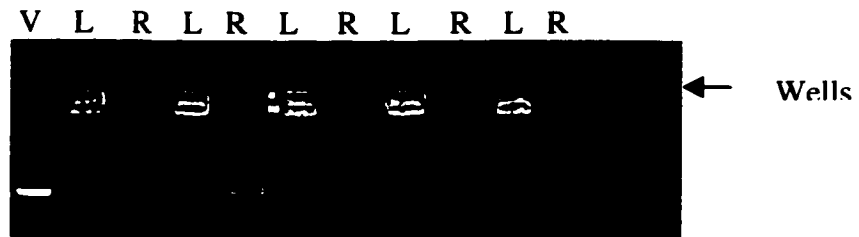
Figure 4. Amount of plasmid DNA present in the recovery chamber after 10 minutes of electrofiltration followed by a 0, 30, 60, 90 and 120 second backward pulse at 250V. Lane V shows the pure vector standard while lanes L are DNA present in the loading chamber after electrofiltration + backward pulse and lanes R are plasmid DNA present in the recovery chamber after electrofiltration + backward pulse.
