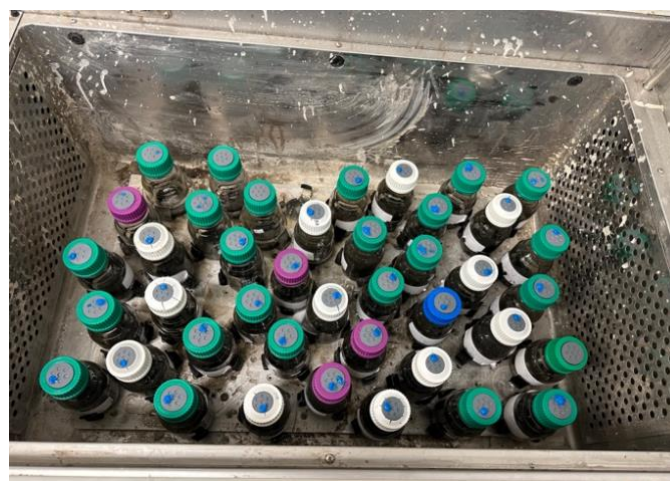
Figure 3.2. BMP bottles with biomass and substrate inside the incubator.
