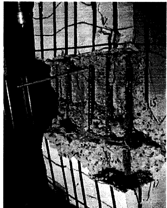
(k) Bars Rupturing
