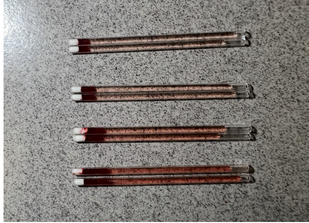
Figure 3.3: Crit Spin micro-hematocrit tubes displaying red blood cell suspensions at various hematocrit (Ht) levels for validation. From top to bottom, the tubes represent 5%, 10%, 15%, and 20% Ht. The packed cell volume in each tube confirms the accuracy of the prepared Ht concentrations for subsequent experiments.
