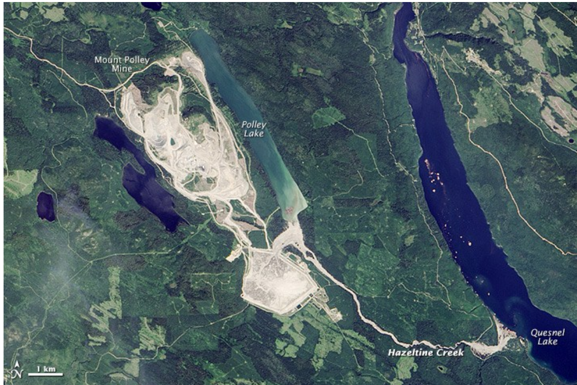
Figure 2-3: Image of Mount Polley from 5 August, 2014, after the dam breach. Image Credit: NASA Earth Observatory images by Jesse Allen, using Landsat data from the U.S. Geological Survey.
