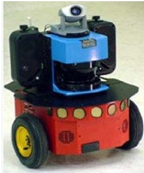
Figure 2.20: Using people detection and laser range sensor to follow a person
