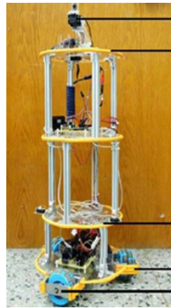
Figure 2.22: Using infrared LEDs to follow a person
