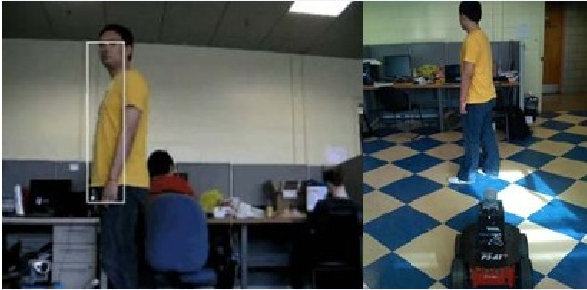
Figure 2.19: Using people detection and laser range sensor to follow a person
