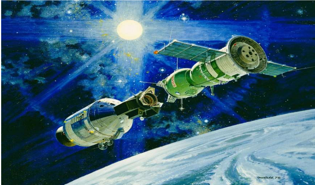
Figure 9 - Artist impression of ASTP. The Docking module is the black part attached to the Apollo spacecraft facing the Soyuz Spacecraft.
