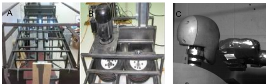
Figure 5. The High-speed impacting system (HSIS) consists of a dual rail system mounted on a steel frame, with a steel carriage for the attachment of the impacting mass (A). The carriage is passed through two spinning wheels powered by an electric motor at a desired velocity (B). The final photo on the left demonstrates the launched anvil simulating a shin-to-head impact (C).
