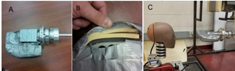
Figure 3. The impacting anvil used to simulate punch, kick, and elbow events (A) with layers of foam attached (B) and impact set-up using the HSIS (C).
