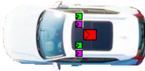
Figure 2.27: Birds eye/top down view of the mounting of sensors to the KITTI data acquisition vehicle. Sensors are color coded (Red: LiDAR, Green: Grayscale camera, Purple: Color camera)
