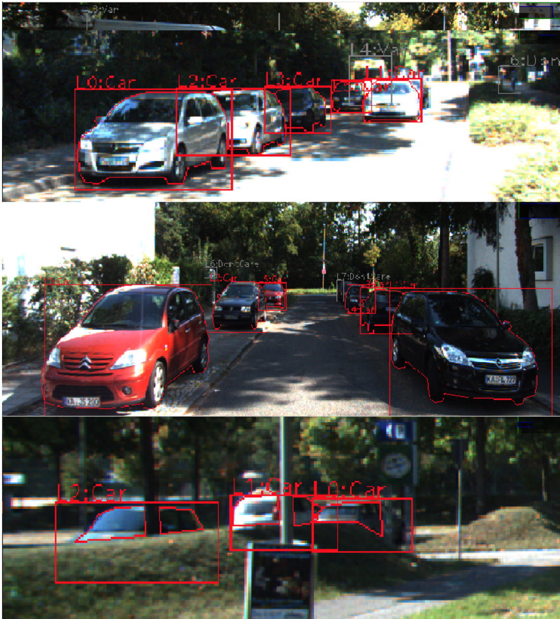
Figure 5.4: KITTI 'Car' class semantic segmentation annotation examples (red boundaries) along with ground truth bounding boxes (images from [37])
