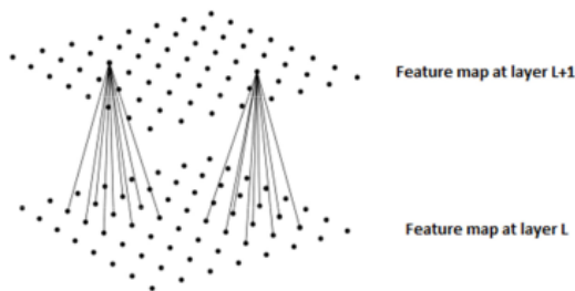
Figure 2.4: Each receptive field is actually just connections to discrete positions in feature maps at the previous layer [107]
