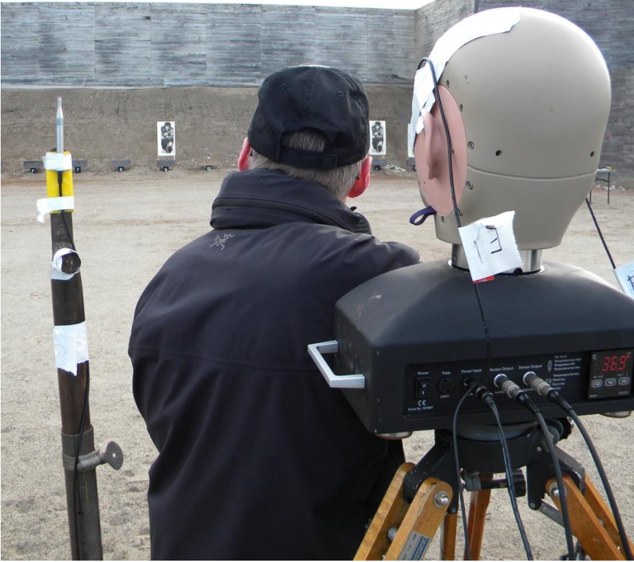
Figure 16 : Impulse Noise Test Setup - Implementation
