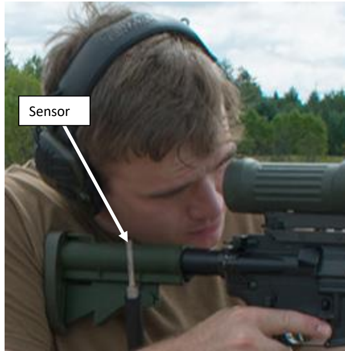
Figure 9: sensor used to measure the exposure level
