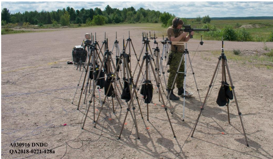
Figure 7: Sound radiations measurement for a small firearm
