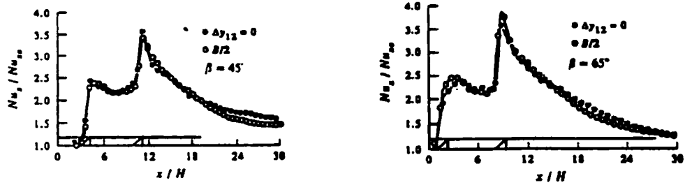
Figure 2.5: Normalized span-average Nusselt numbers for in-line ( \Delta y_{12}=0 ) and staggered ( \Delta y_{12}=B/2 ) winglets, adapted from Tiggelbeck et al. (1993) with permission of ASME.
