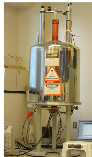
Figure 2.2.4. Bruker AVANCE III 200 NMR spectrometer instrument used in this study.
