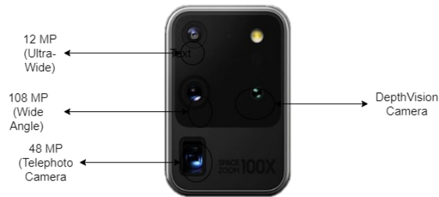
Figure 5.1: Schematic demonstrating the camera of the Samsung S20 Ultra 5G Smartphone used for data collection.
