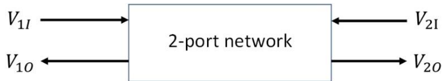
Figure 4: Graphic representation of a 2-port network where V_{1I} and V_{1O} are the input and output voltages of port i , respectively.
