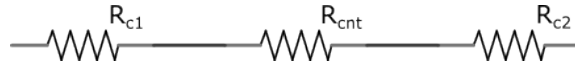
Figure 4.2: Sample resistive model where R_{c1} and R_{c2} are the CNT-Paperclip connection resistances and R_{cnt} is the resistance of the fibre.
