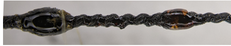
Figure 3.11: Damaged sample after exposure to a 2.5 V for 5 s , resulting in epoxy discolouration and reduction along the centre portion of the sample. Globes at the ends are exaggerated due to the resetting of the epoxy at the increased liquid state.
