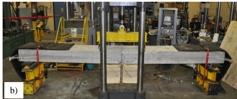
Figure 4-4 a) Test setup schematic, b) Full-scale test setup (Noël, 2013)
