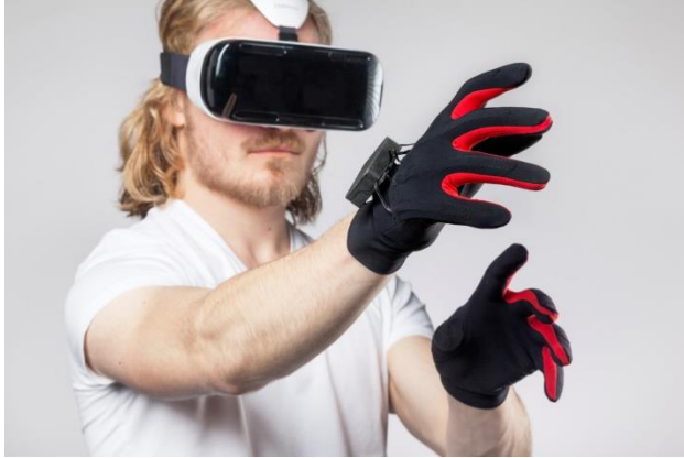
Fig 2-3. VR haptic gloves. Peripherals that can be used alongside VR headsets to provide users with tactile feedback and a more immersive experience [78]
