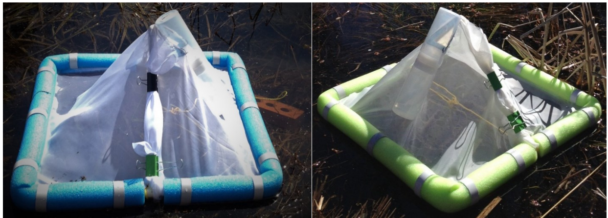
Figure 2. Insect emergence trap design is framed with a PVC-skeleton, draped with fine transparent netting that directs insects into the collection cup opening at the top of the frame. The collection cup holds 100-150 mL of 70% isopropanol as a preservative. Polyethylene foam allows the trap to float while tethered by an adjustable rope and anchored by a brick.
