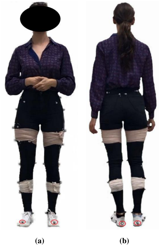
Figure 5.10 (a) Front and (b) back views of a participant with reflective markers
