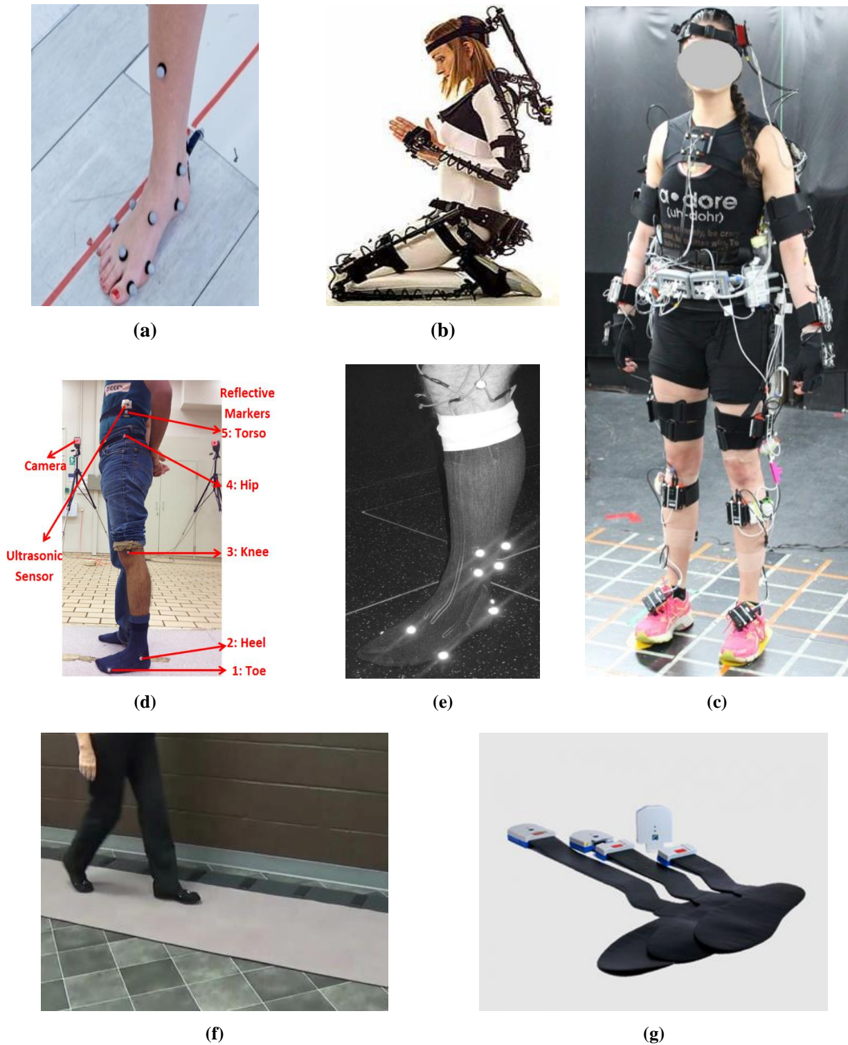
Figure 2.2 (a) Markers for Vicon system (optical motion capture) [20], (b) Electro-mechanical motion capture system [25], (c) Inertial motion capture technology [23], (d) Ultrasonic acoustic technology [26], (e) Instrumented sock [28], (f) GAITrite carpet [29], (g) Instrumented insoles [30].
