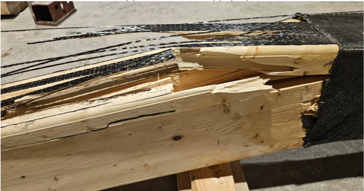
(c) Tearing of tensile unidirectional fabric of G-T(0)M( \pm 45 ) Figure A.16 Static test of G-T(0)M( \pm 45 )
