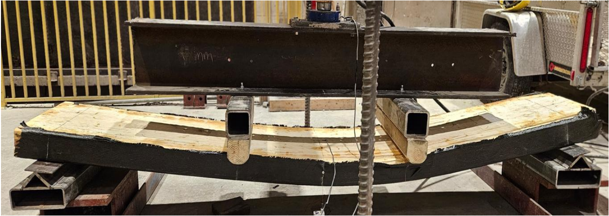
(a) Static failure mode of CLT-T(0)U( \pm 45 )
