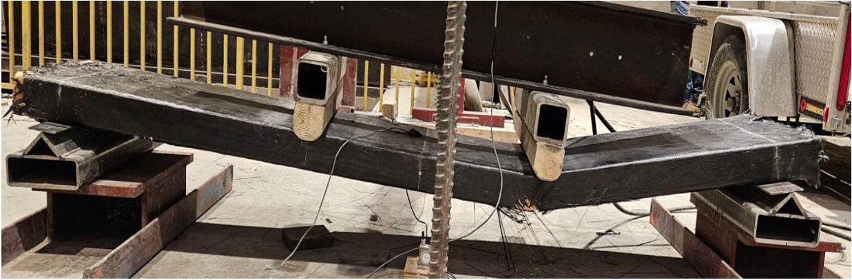
(a) Static failure mode of CLT-T-M(0)C( \pm 45 )
