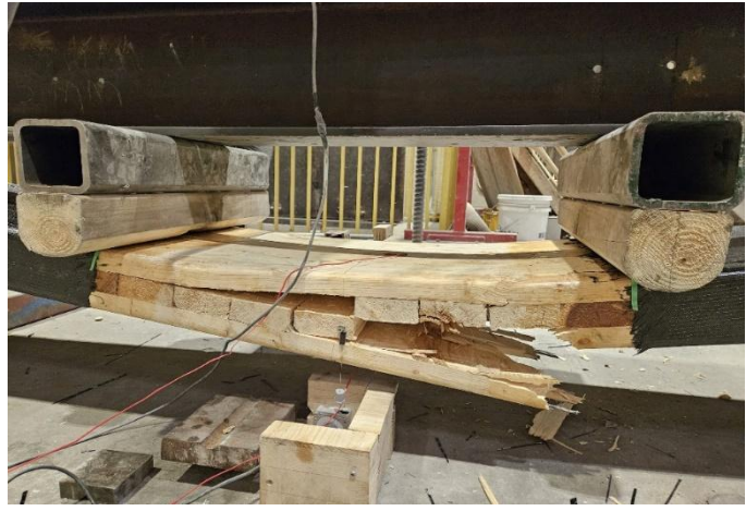
b) Static test CLT-T(0)SH(±45)-1 (outer wood tension laminates with damage)
