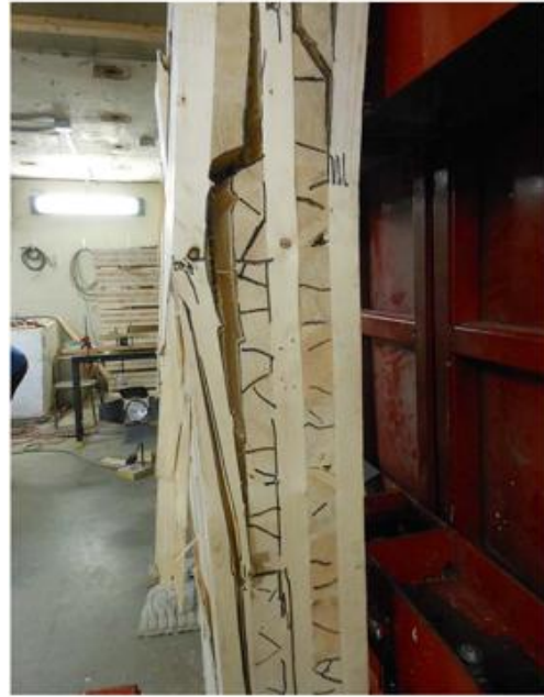
(b) failure of a 5-ply panel (CLT5-4.1)
