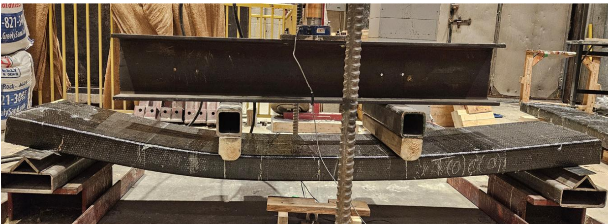
(C) Static failure mode of CLT-T(0)C(0)-2
