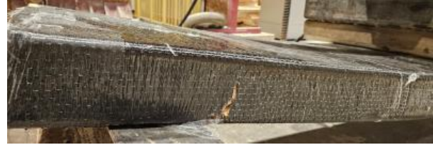
c) Tearing of unidirectional fabric of CLT-T(0)C(0)-2
