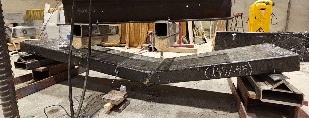
(a) Static failure mode of CLT-C( \pm 45 )
