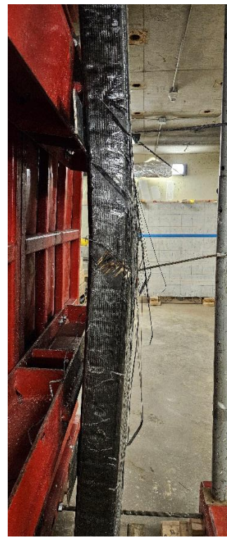
d) Side view of tearing of fabric
