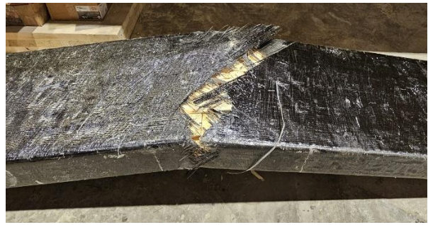
c) Tearing of CFRP reinforcement CLT-C(±45)
