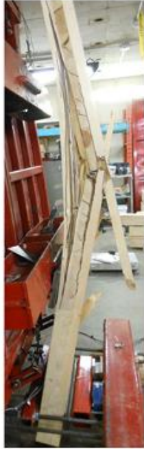
(a) failure of a 3-ply panel (CLT3-5.1)
