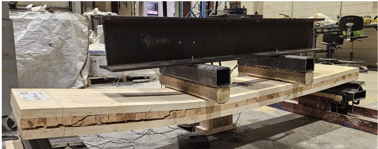
Figure 4.3 Representative static failure mode for unretrofitted CLT panel
