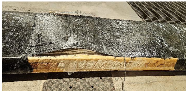
c) Longitudinal Shear in CLT-T(0)SH (±45)-2
