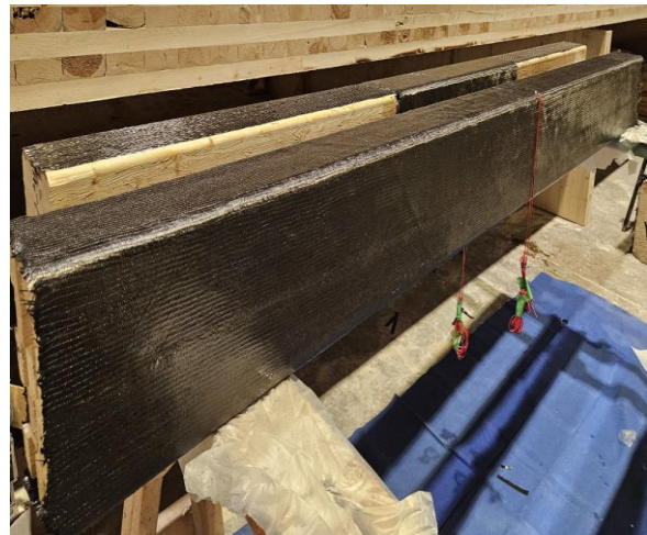
d) Full-length and partial-length confinement of CFRP before curing (Glulam beams)
