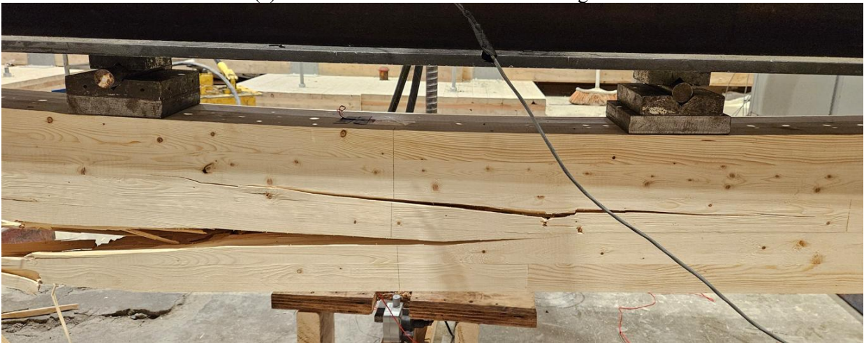
(b) Close view of G-T(0)C( \pm 45 ) between to concentrated loads Figure A.14 Static test of unretrofitted glulam
