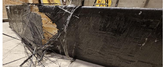
b) Tension side of CLT-T 2 (0)C(±45)
