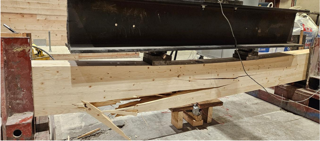
(a) Static failure mode of unretrofitted glulam
