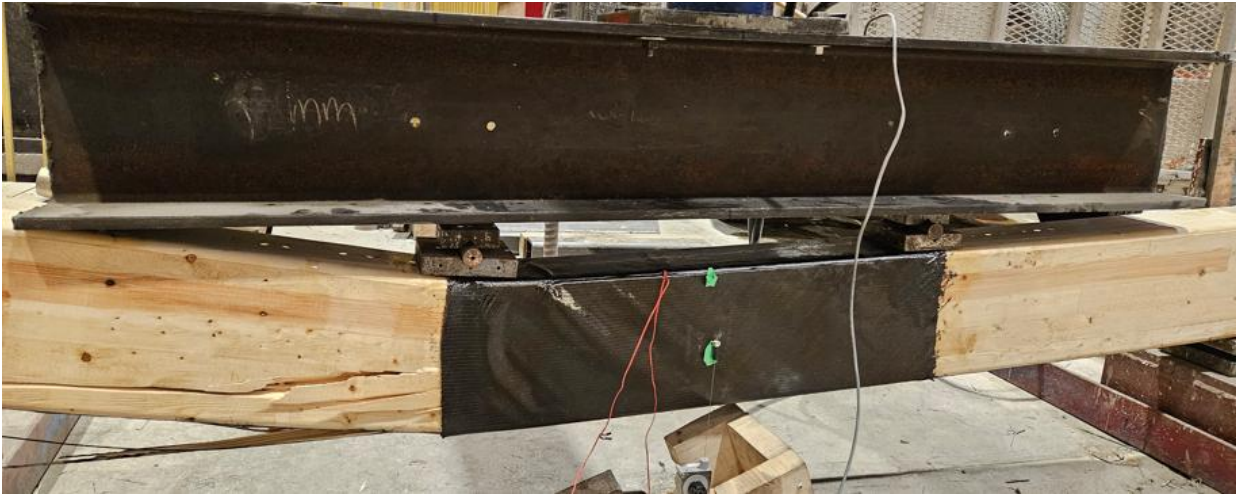
(a) Static failure mode of G-T(0)M( \pm 45 )
