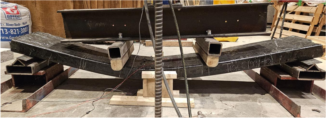
(a) Static failure test of CLT-T(0) 2 C(±45)
