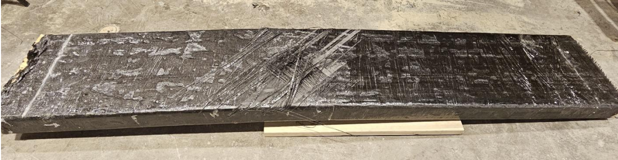
c) Tension side of CLT-T-SH-M(0)C(±45)
