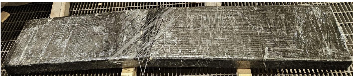
(b) Tension side of CLT-T(0)C(±45)-2
