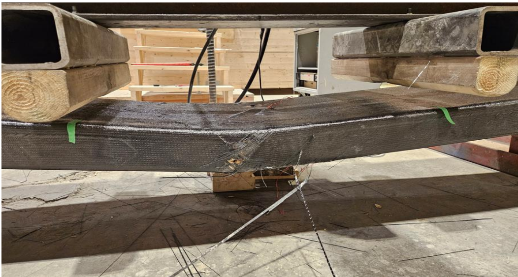
(b) Close view of CLT-T(0)C( \pm 45 )-1
