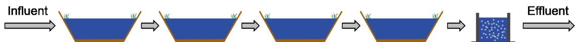
Figure 7.3 Simplistic design representation of a post carbon removal nitrifying MBBR at the Masson Angers lagoon treatment wastewater treatment plant
