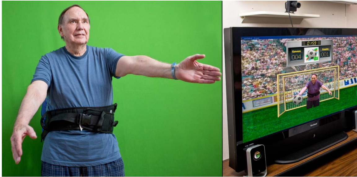
Figure II: VRRASS participant playing the soccer application. LEFT: Participants stood in front of a green screen with a physio belt around their waist while being monitored by a researcher (behind the participant). RIGHT: The participant sees himself immersed in a soccer net. Above the TV is the camera that captures the image of the participant. Photo used with permission of the participant.
