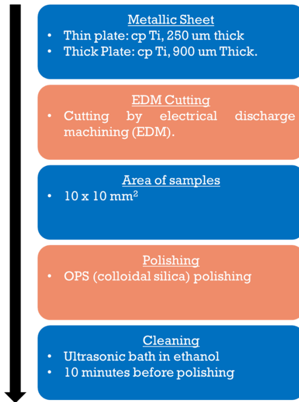
Figure 3-1 Flow chart describing procedures of pre-treatment before laser texturing on Ti.
