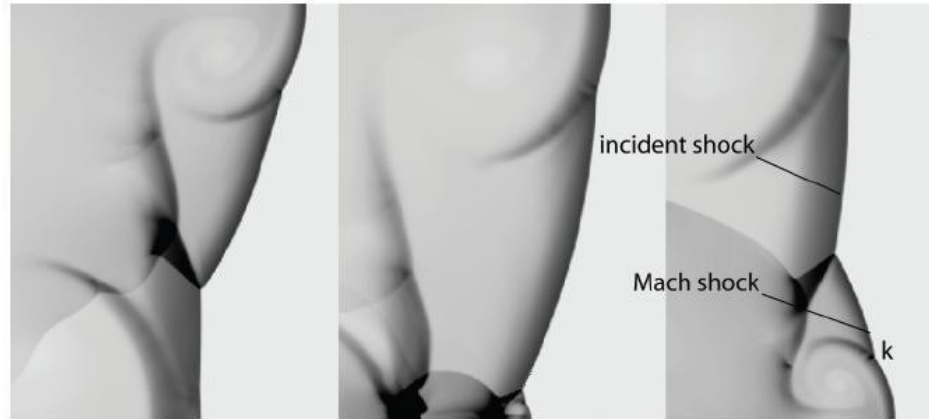
Figure 7: Three consecutive density plots of a numerical simulation of a detonation ( \gamma=1.2 , Q/RT_0=50 , and Ea/RT_0=27 ). A bifurcation (labelled k) can be observed after the triple point reflects off the lower wall. Taken from Radulescu (2007).
