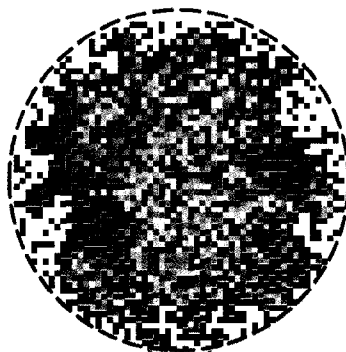
FIGURE 4.1 Optimized hydrogel of radius r_0 = 31 . The obstacles are in black and the initial drug concentration is shown ranging from low (blue) to high (red). The outer boundary of the hydrogel is schematically shown as the grey dashed line. Notice all the familiar structures found in the previous optimizations. Namely, the creation of an obstacle boundary somewhere in the hydrogel and a high concentration of drug near the centre to help curtail any strong initial drug peak.
