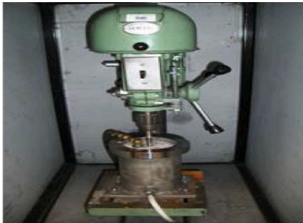
Figure 3.2: Custom-made attritor mill.
