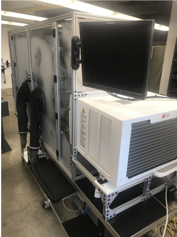
Figure 4 - Enclosure featuring the newly added air conditioning.
