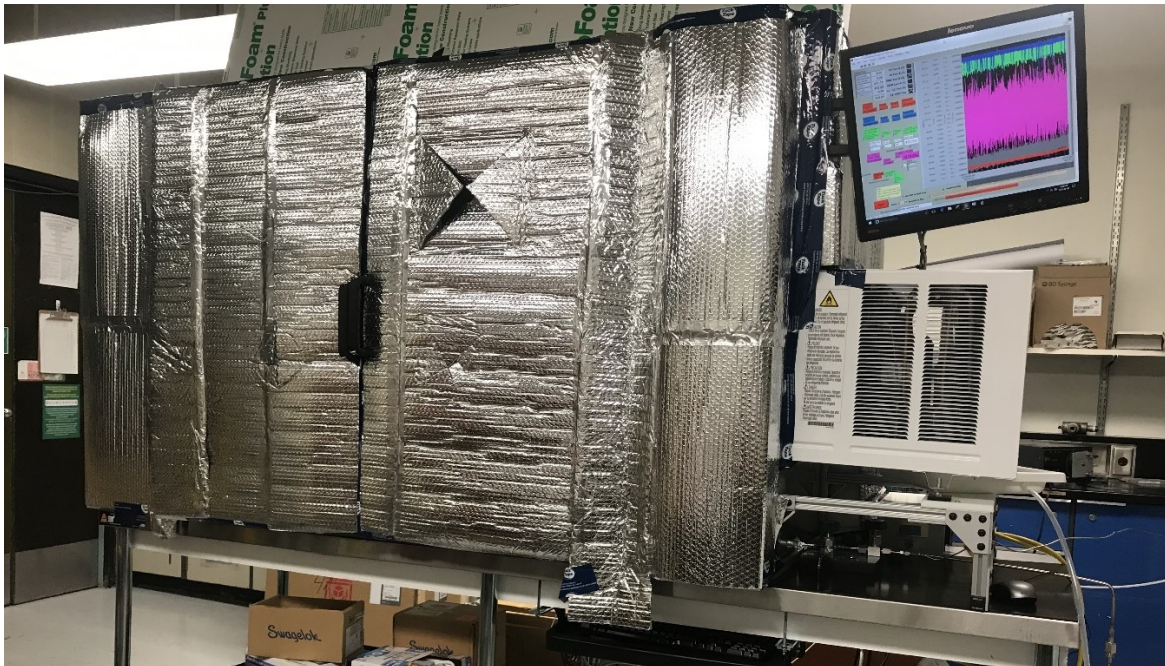
Figure 5 - Insulated enclosure with heating and cooling capabilities.
