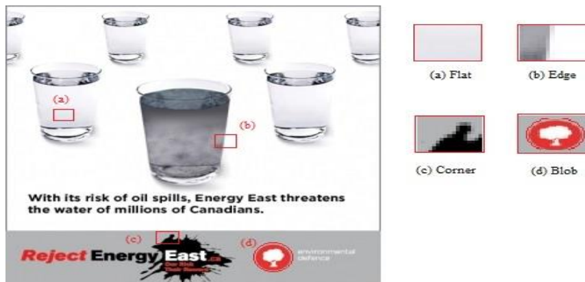
Figure 2. Extracting different feature types from an image: (a) flat, (b) edge, (c) corner, and (d) blob
