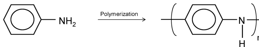
Figure 10-1- Schematic picture of aniline monomers ( C_6H_7N ) and polyaniline ( (C_6H_7N)_n )
