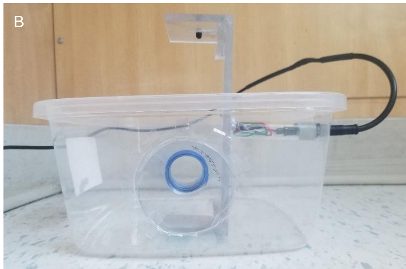
Figure 18. Phonotaxis test apparatus, described in Section 3.5, Figure 14. A) Bird's eye view and B) front view of trap with C) infrared sensor.
