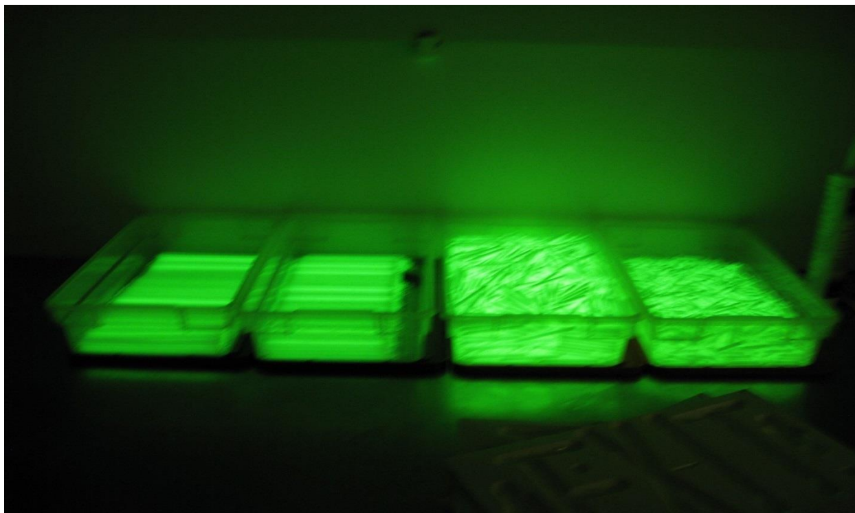
Figure 5: Tritium encapsulated in Beta-light vials at SRB Technologies, Pembroke, Ontario, Canada.
