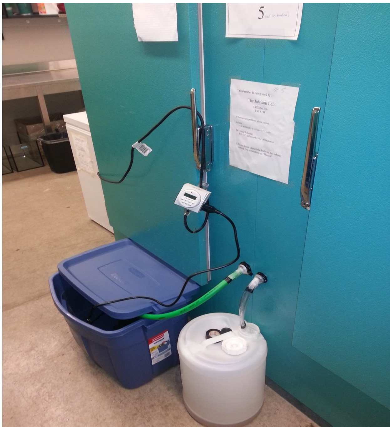
Figure 7: Growth Chamber Conviron growth chamber with water reservoir supplying the plants inside. Drainage is discharged into the white barrel.
