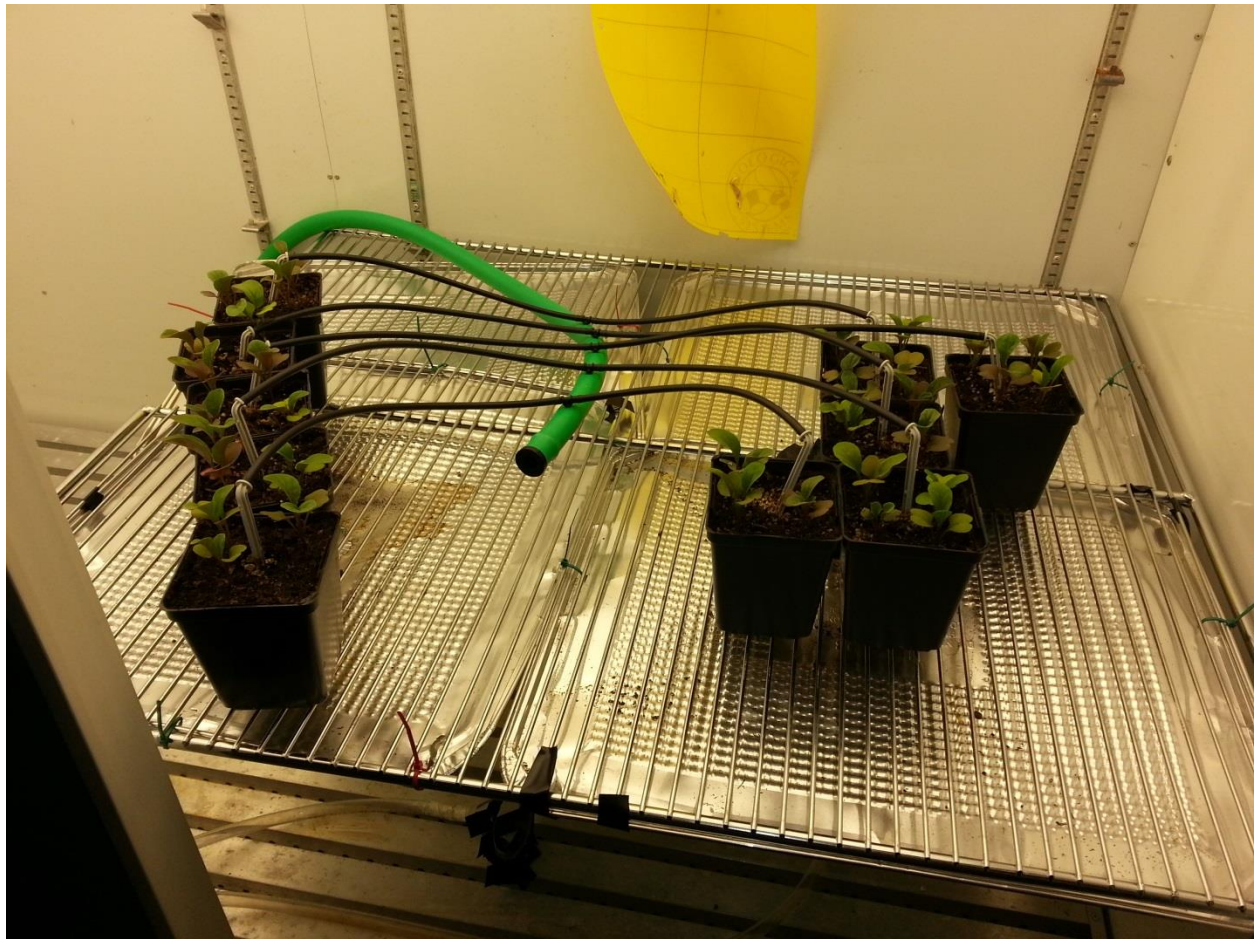
Figure 8: The scheduled hydroponic drip system provided water to the plants three times a week to maintain consistent growing conditions. Note that there are several seedlings per pot. This was later changed to increase leaf volume, as plants grown in close proximity led to reduced growth.
