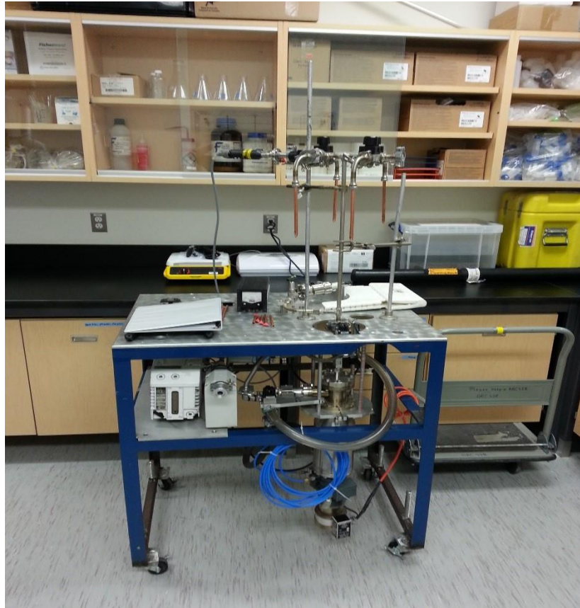
Figure 15: Helium ingrowth preparation line. Samples are packed tightly into copper tubing, then the air is evacuated in each tube using a diffusion pump. At the appropriate vacuum pressure, the tubes are crimped and left to accumulate helium from tritium decay.
