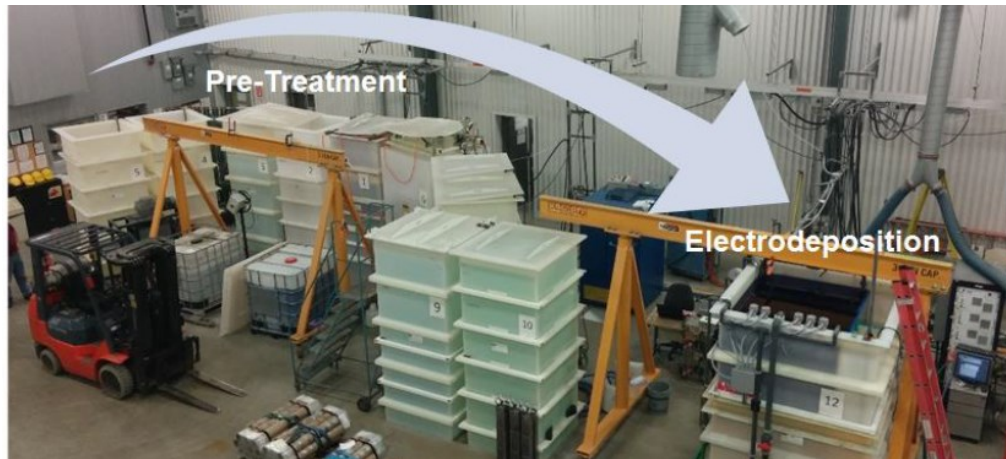
Figure 2.10 Copper electrodeposition pre-treatment and process [8].
