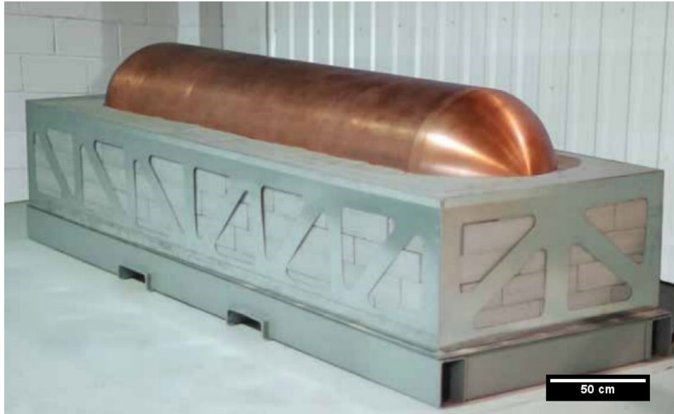
Figure 2.6 UFC inside the bentonite clay buffer box [1].
