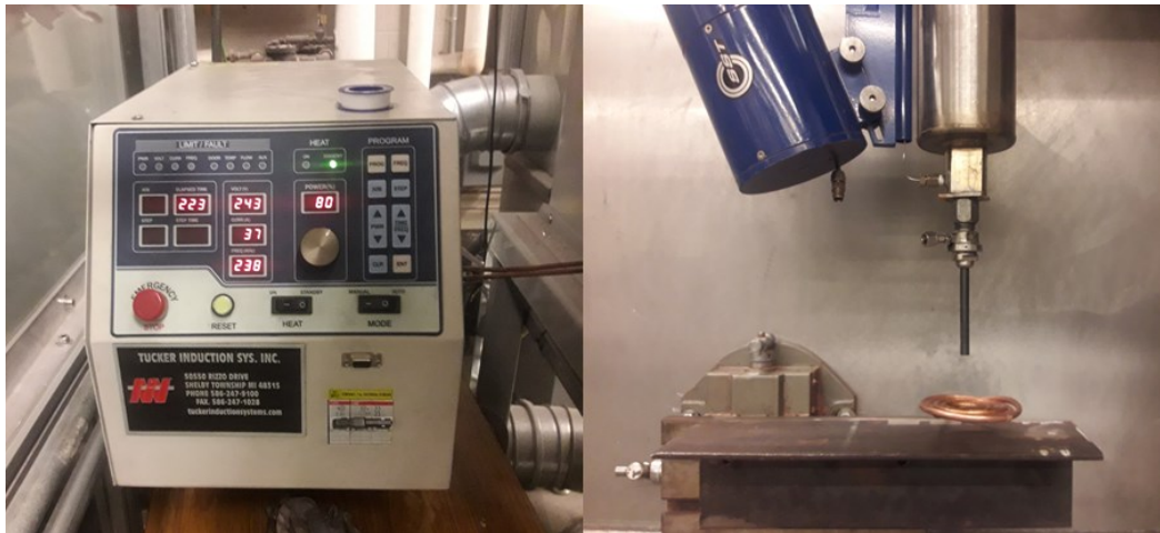
Figure 4.17 Induction heater machine (left) and final coil set up inside the CGDS chamber (right).
