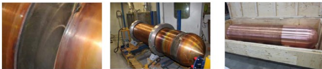
Figure 2.9 Full-sized leading assembly: close-up of closure weld area after welding and machining (left), installed with collars on roller frame before the coating of the closure weld (middle), and (c) after coating and machining of the closure weld (right) [8].
