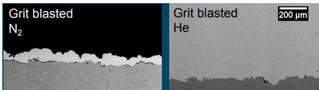
Figure 2.13 SEM Cross section image of the interface copper coating with low carbon steel substrate preparation of grit blasted with N_2 (left) and He (right) as carrier gas [23].
