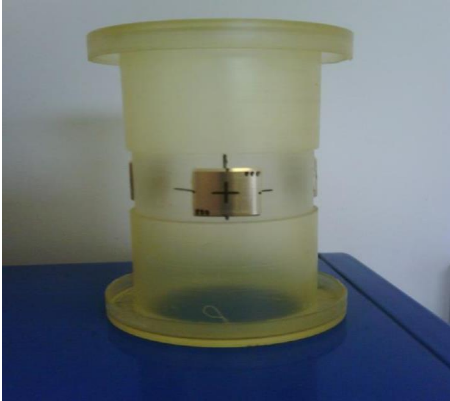
Figure A.13 Modified Hoek sleeve with brass additions (Cuss et al., 2012)
