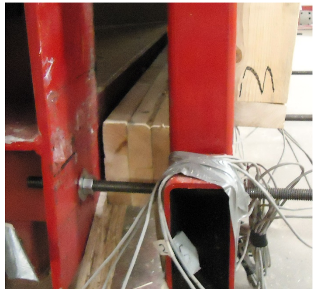
d) Lateral displacement due to bottom connection failure
