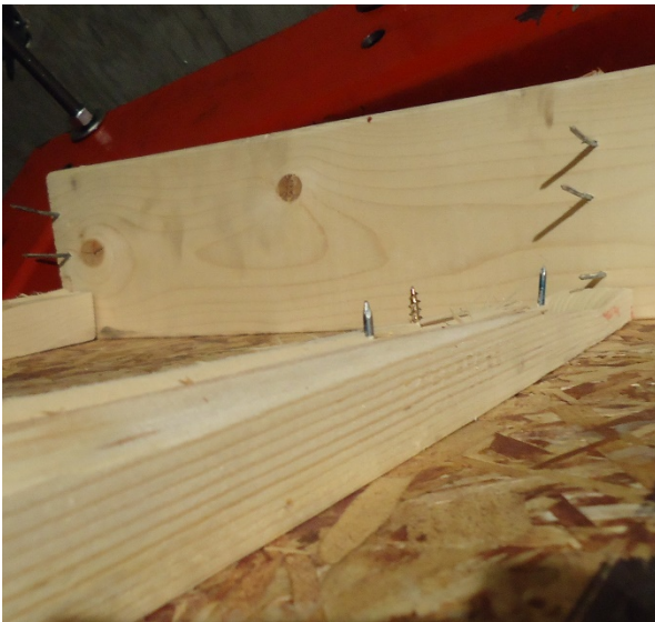
b) Exposed fastener tips along failure zone of Stud 5
