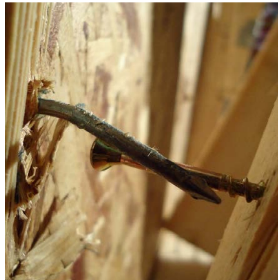
B. Nail withdrawal and screw head pull-through
