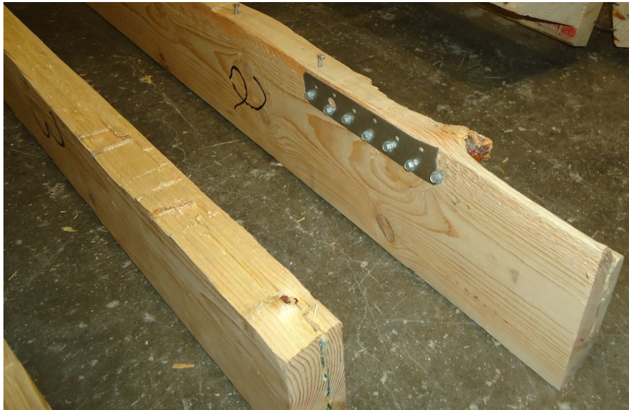
c) Rupturing of LTS18 connector on Stud 2
