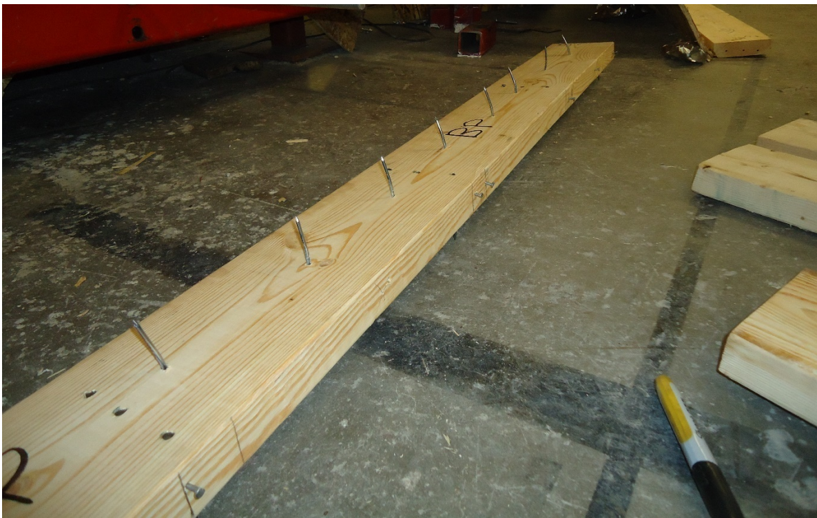
c) Nail withdrawal at bottom plate
