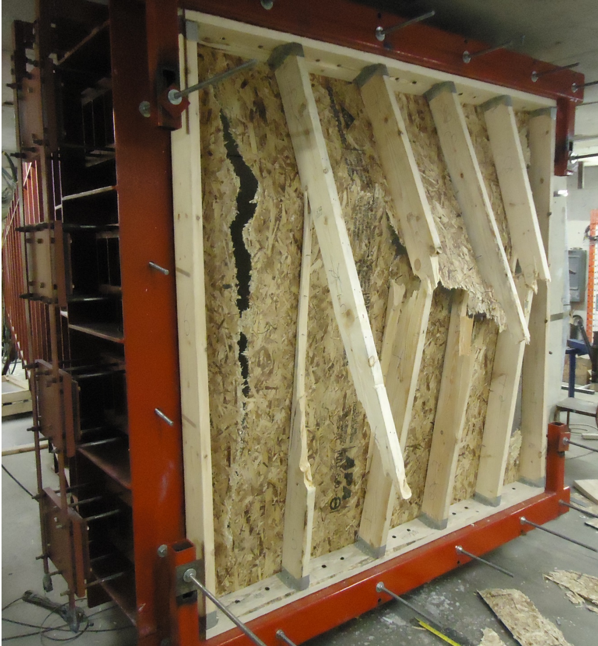
Figure 6.15 : Wall 20 detailed with HU28 connectors
