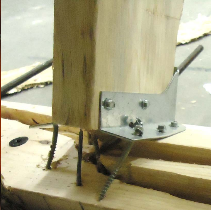
b) HU28 fastener withdrawal
