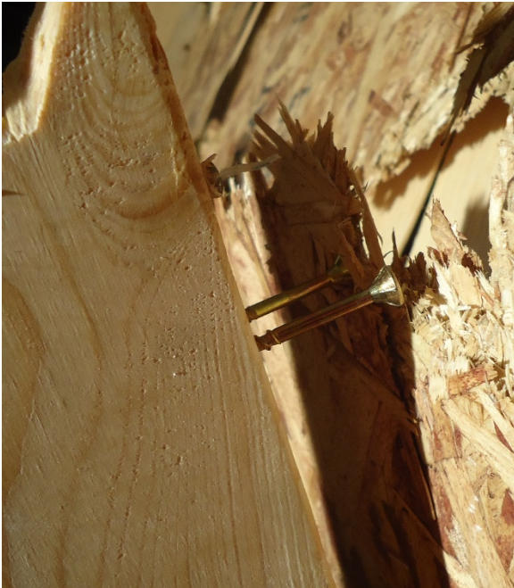
b) Nail and screw head pull-through
