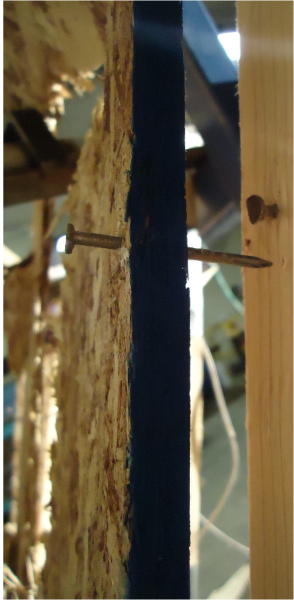
c) Nail withdrawal and head pull-through
