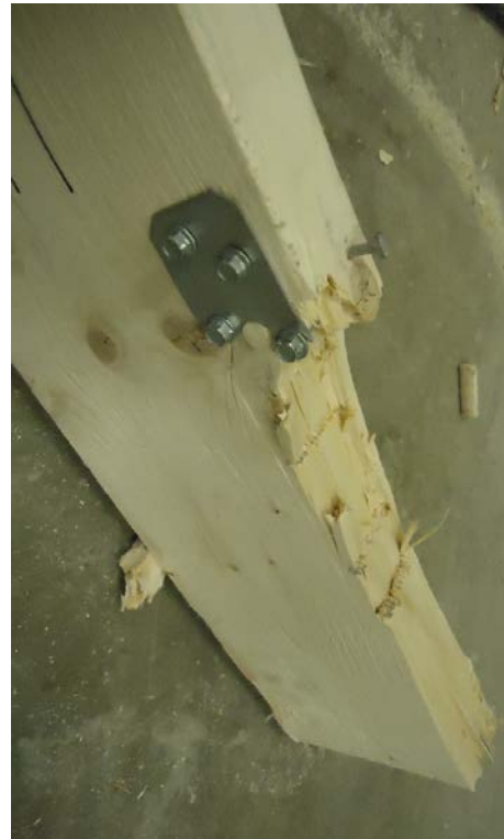
B. Combined rupture/splitting failure
