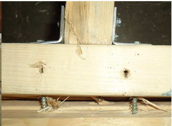
d) HU28 fastener withdrawal
