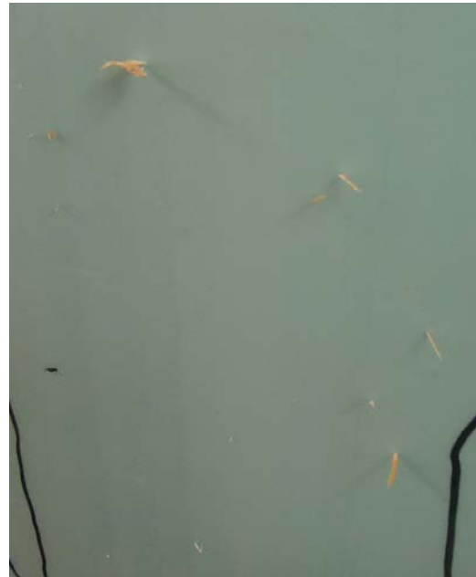
B. Splinters embedded in Polystyrene panel
