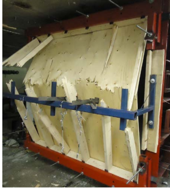
B. Plywood wall with failed studs missing from specimen
