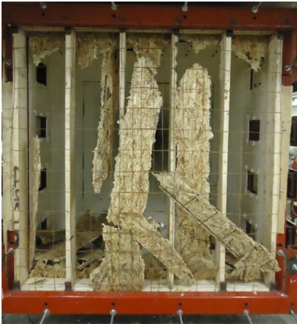
A. Control of sheathing debris
