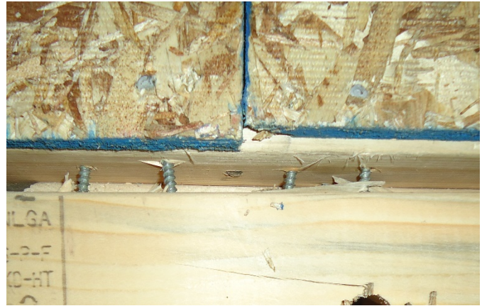
d) Slight LJS26DS fastener withdrawal
