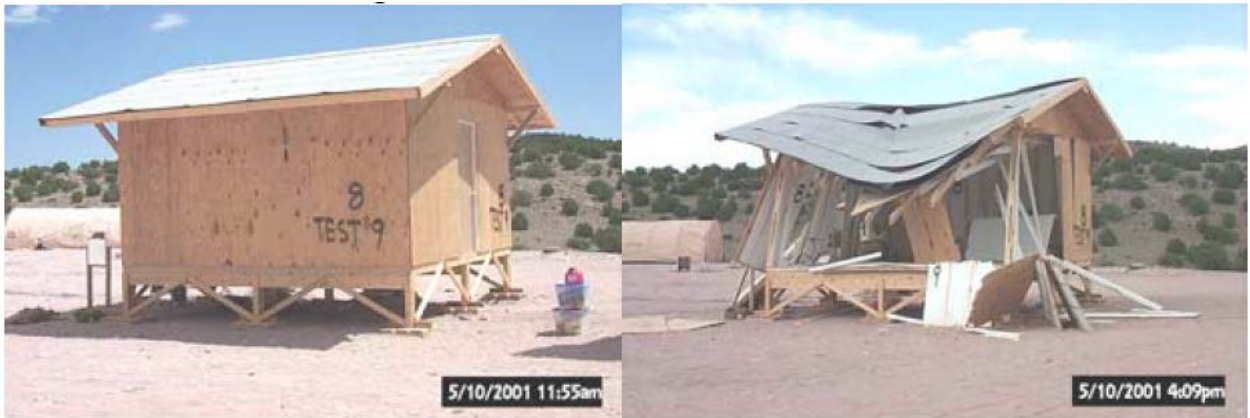
Figure 2.2 : SEA hut before (left) and after (right) testing (USAF, 2006)
