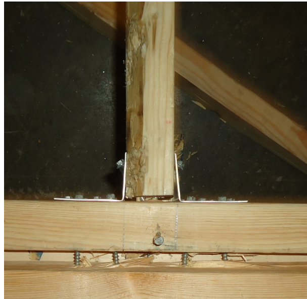
d) Slight LJS26DS fastener withdrawal
