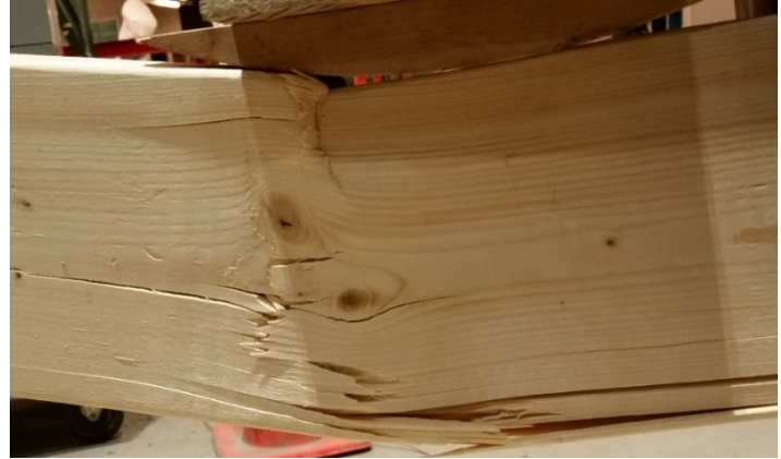
B. Crushing of wood fibres and tension failure
