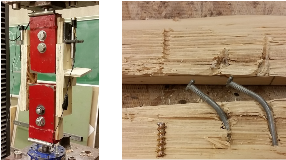
Figure 3.9 : Typical test setup and failure mode for load-slip tests
