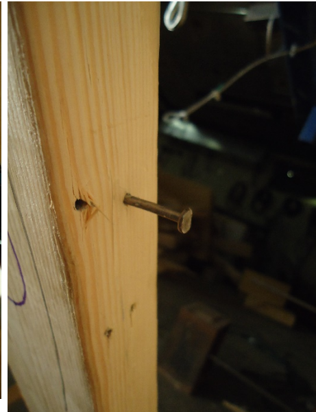
d) Nail head pull-through
