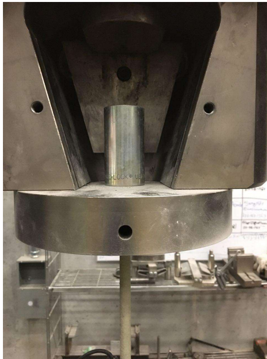
Figure 3.9 Top Head, Anchorage Pre-Stressing Wedge System
