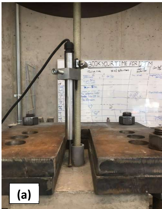
Figure 3.10 LVDTs Attached to: (a) Top; (b) Bottom
