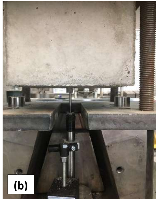
Figure 3.10 LVDTs Attached to: (a) Top; (b) Bottom
