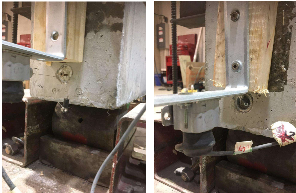
Figure 4.11 Unloaded End Slippage; (a) Before Slippage, (b) After Slippage
