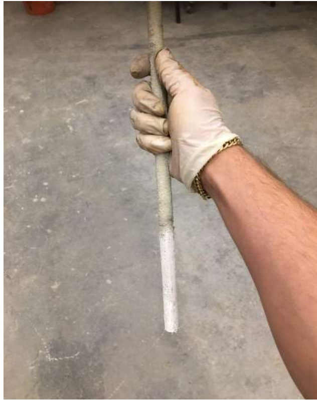
Figure 3.12 Bar Deformation after Pullout
