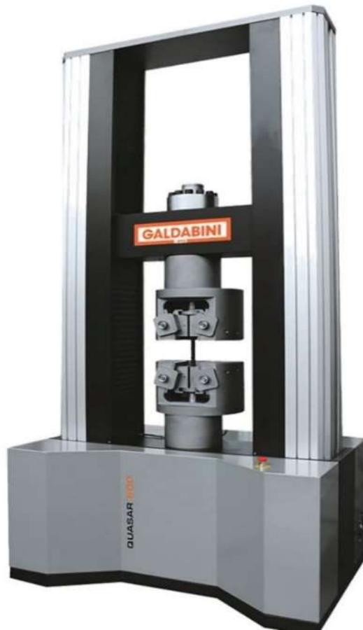
Figure 3.6 Universal Testing Machine
