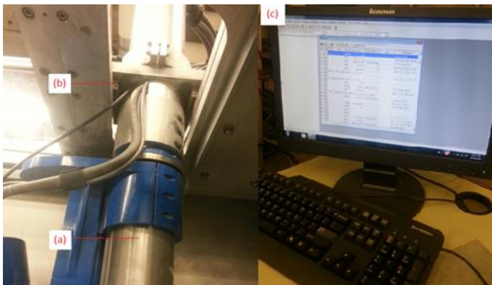
Figure 4.3: a) X-Y robot, b) spray gun c) X-Y robot interface
