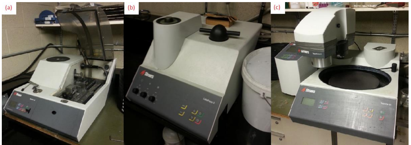
Figure 4.9: Equipment used to prepare samples prior to analysis, a) Cut-off saw (Struers Secotom-10), b) Epoxy resin mounting equipment (Struers LaboPress-3), c) Polishing apparatus (Struers Tegrapol, TegraForce-5 and TegraDoser-5)
