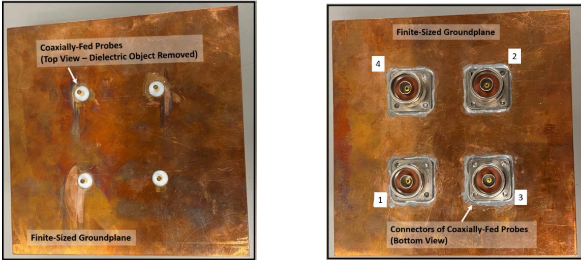
Figure 3.7-3: Top view of finite-sized groundplane (left), with DRA removed, showing the four probes, and bottom view (right) showing the four coaxial connectors.
