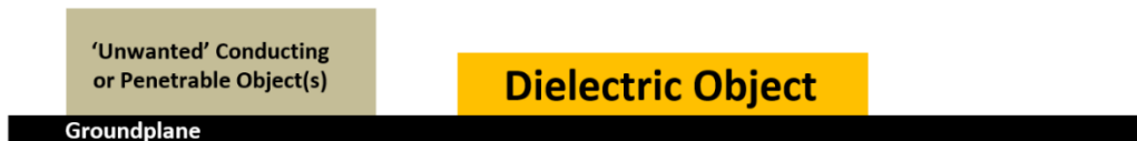
Figure 3.6-3: Situation for CM computation for a dielectric object in the presence of another object, both located on a groundplane.
