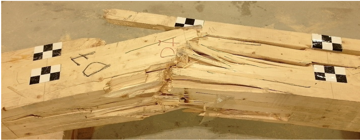
Figure 4.22: Failure of specimen D-20M-B1.
