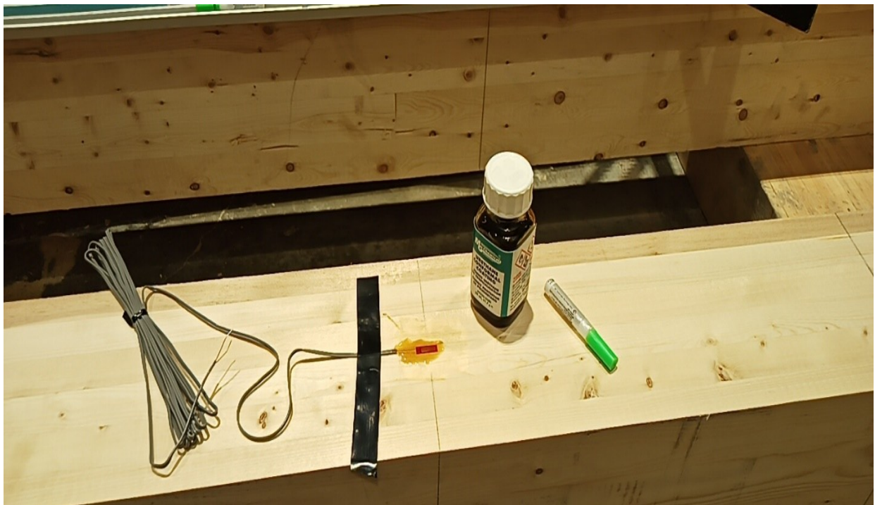
Figure 3.6: Strain gauge application (wood).
