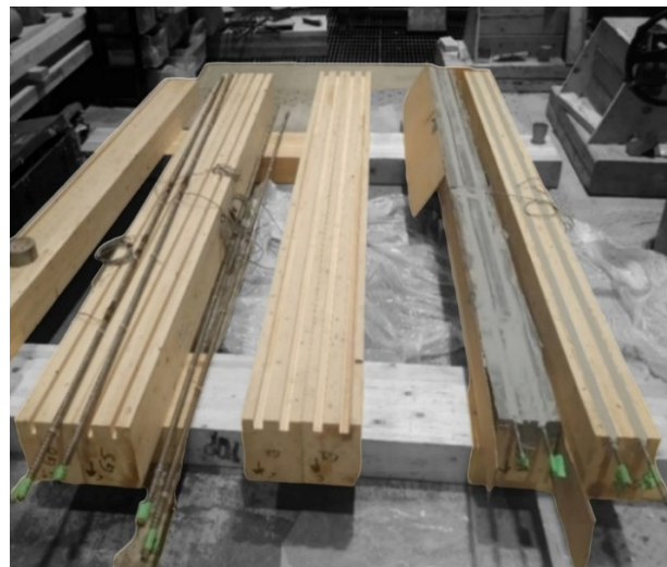
b) Beams under reinforcement
