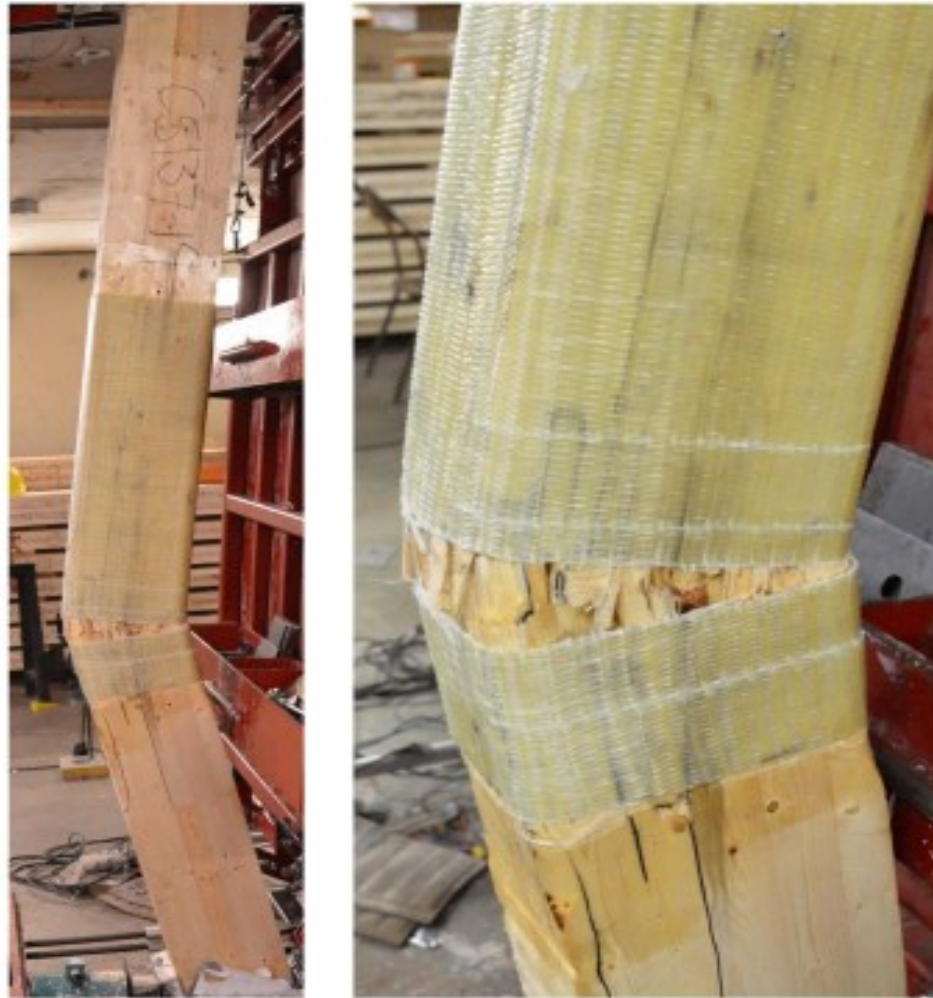
a) Reinforced beam b) Close-up for mid region
