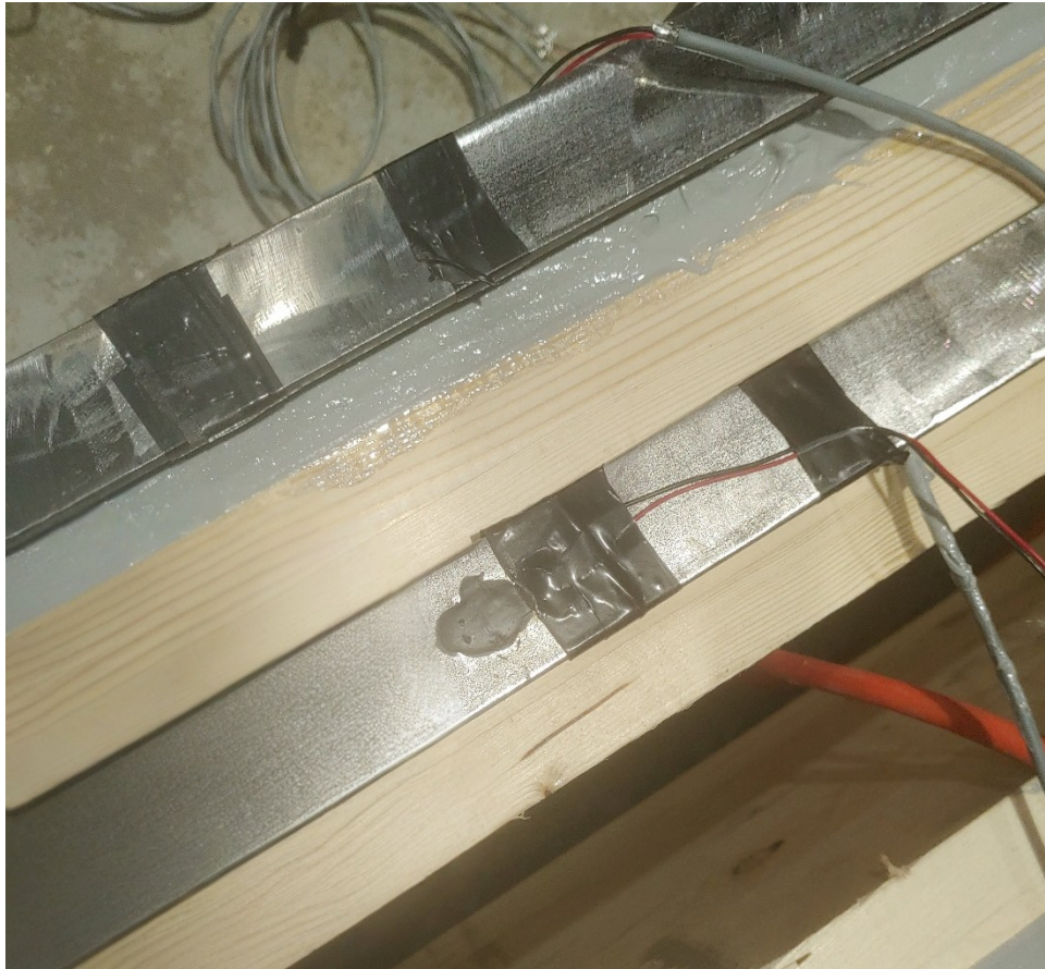
Figure 3.7: Strain gauge application (steel).
