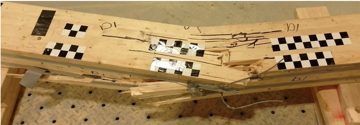
c) Damaged beam
