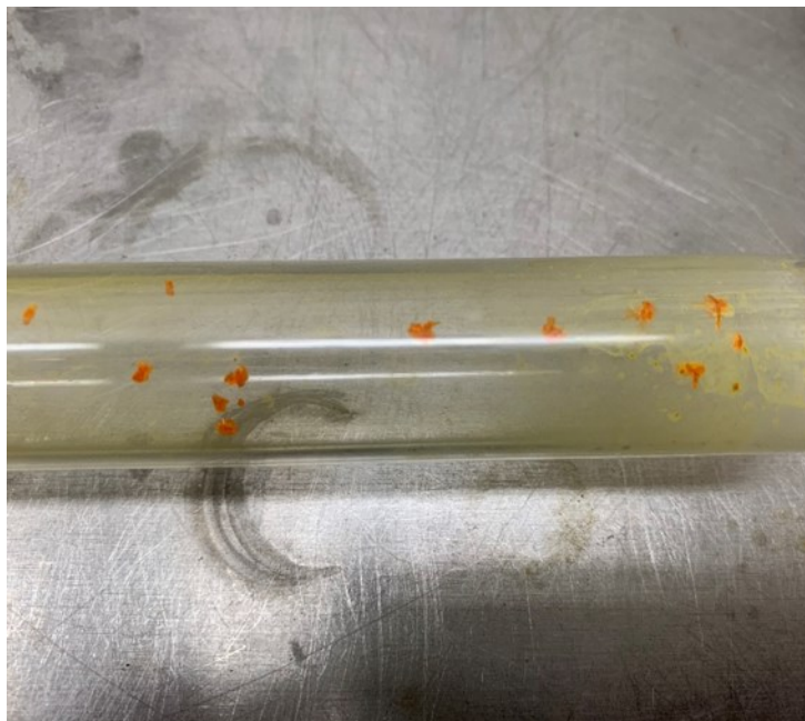
Figure S 19. Orange \text{Br}_2 \cdot \text{TMP} cocrystals (3) obtained using a cosublimation furnace.
