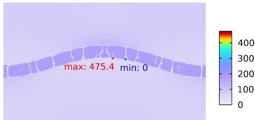
Figure 25: Distribution of von Mises stress in the damaged TGO layer, showing stress relaxation due to fracture.
