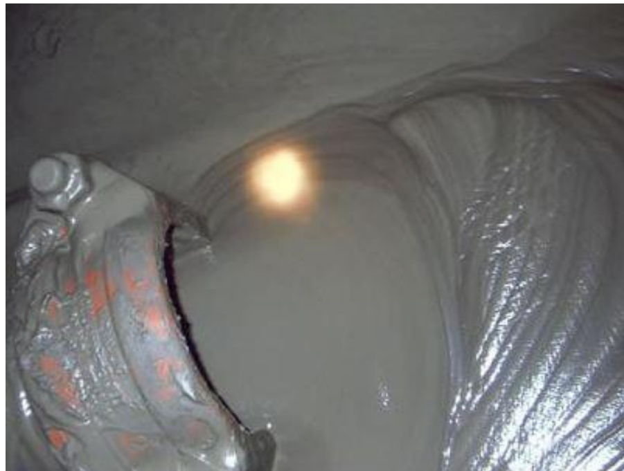
Figure 2.4: Sample of hydraulic backfill (O'Toole, 2004)
