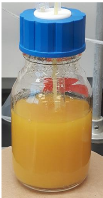
Figure 3-5: Aqueous slurry of \text{As}_2\text{O}_3 reacted with \text{H}_2\text{S} (g).
