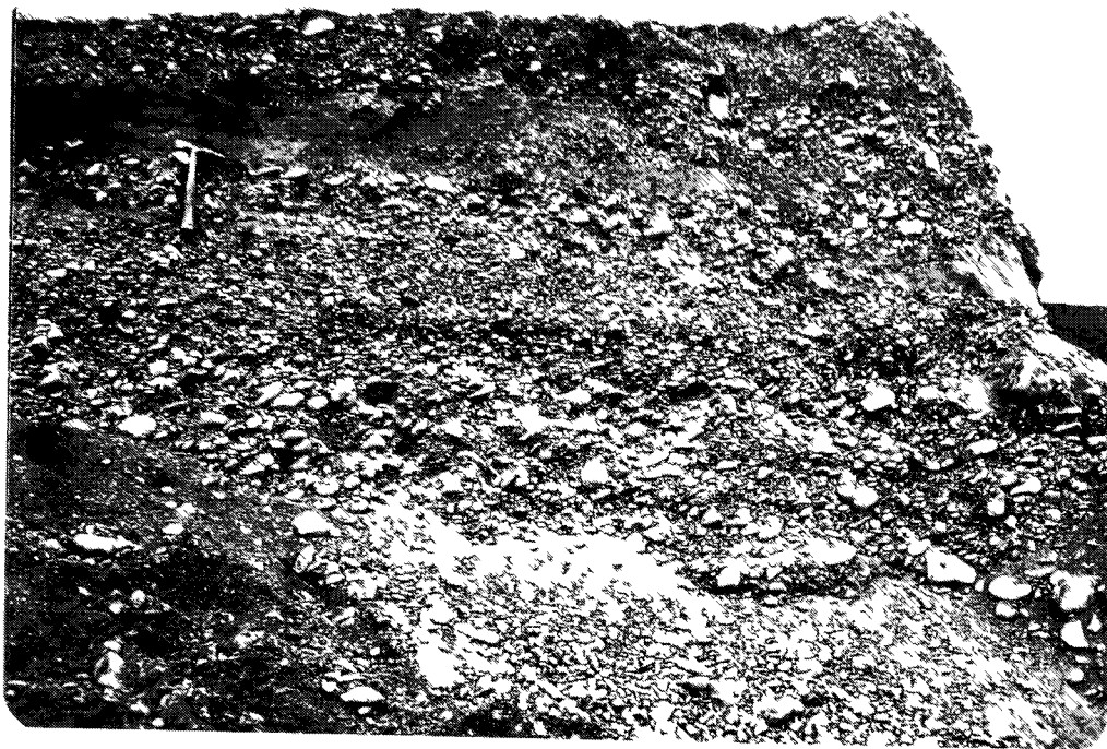
Plate 23. Planar cross bedded gravel (Gp) and fines (F1, Fm) in member C of the Klondike Gravel (JC3).
