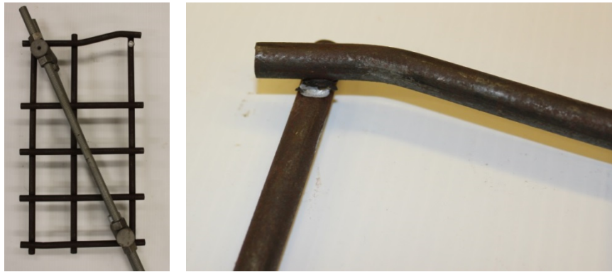
Figure 4.16 Burst Test – Failed 8-Cell Grid
