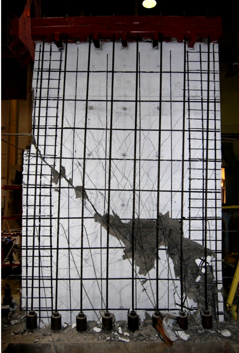
Figure 5.12 (Cont'd) Shear Wall No. 1 Failure Photos
