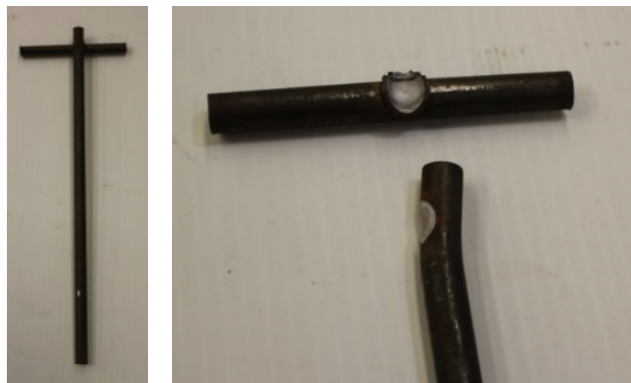
Figure 4.3 WWR Grid Joint Specimen (Left); Failed Specimen (Right)
