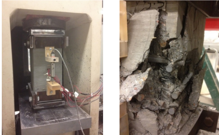
Figure 4.32 Small Scale Column Test Setup (LEFT) and Failed Specimen (RIGHT)
