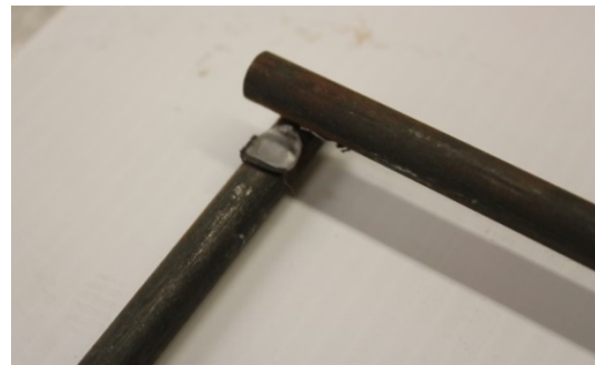
Figure 4.14 Burst Test – Failed 3-Cell Grid
