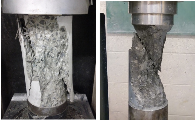
Figure 3.3 Concrete Cylinder Sample under Axial Compression
