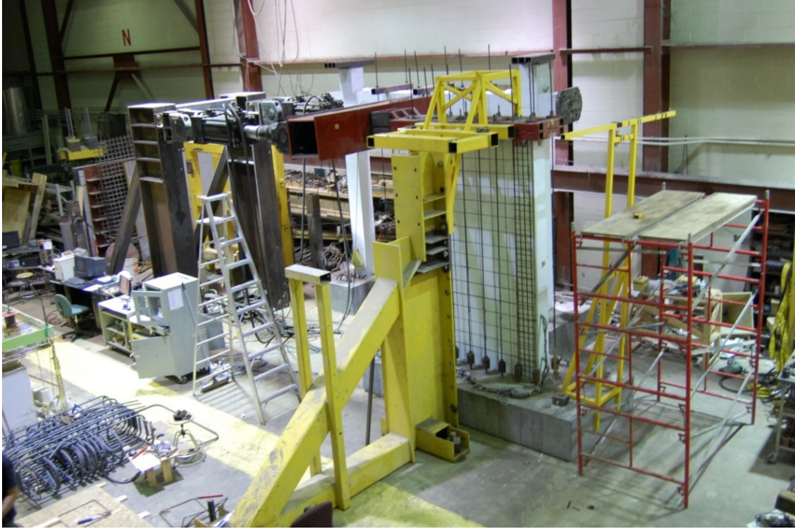
Figure 5.20 Shear Wall No. 2 Test Set-up
