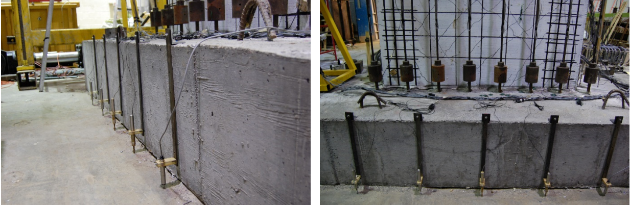
Figure 5.29 Shear Wall No. 2 – Monitoring of Foundation Vertical Movement During Testing
