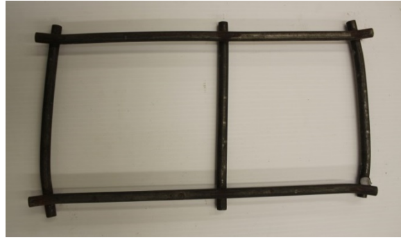
Figure 4.12 Burst Test – Failed 2-Cell Grid
