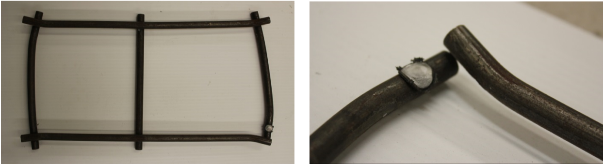
Figure 4.7 Direct Shear Test – Failed 2-Cell Grid
