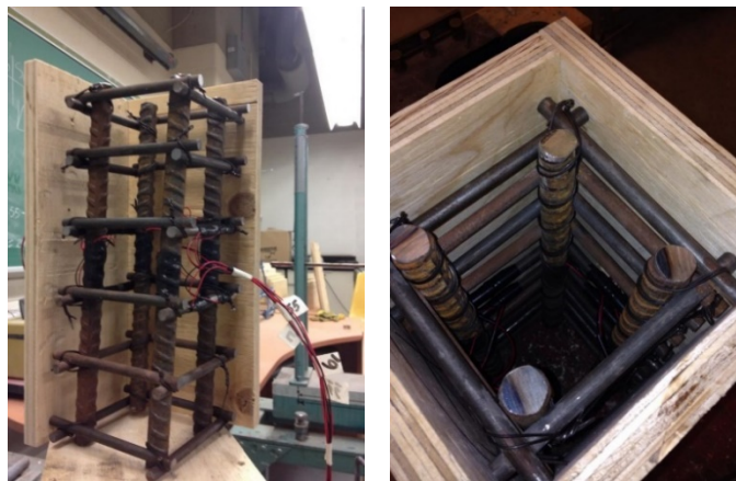
Figure 4.31 Manufacturing of Small Column Specimens
