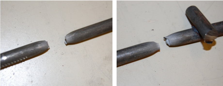
Figure 3.13 Close up Image of Necking of Coupons with and without Welded Segments
