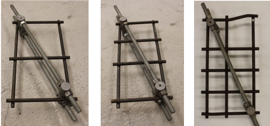
(a) 2-Cell; 3-Cell and 8-Cell Grid Configurations
