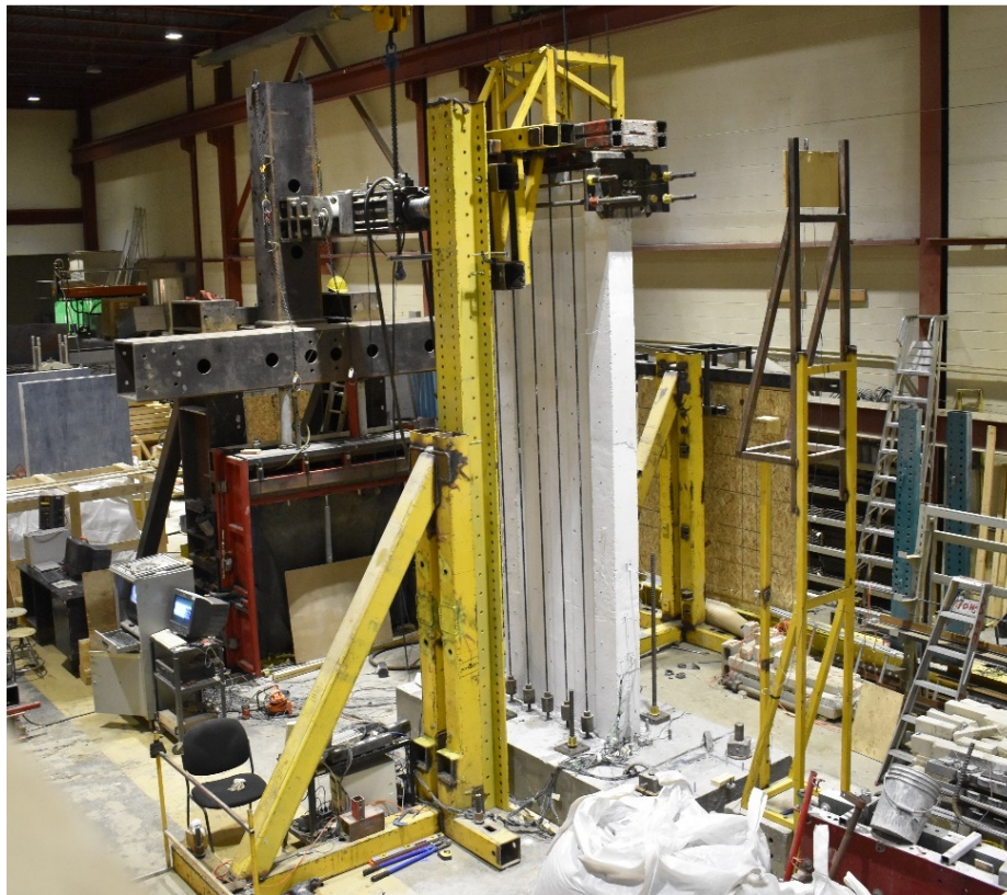
Figure 5.35 Shear Wall No. 3 Test Set up Overview
